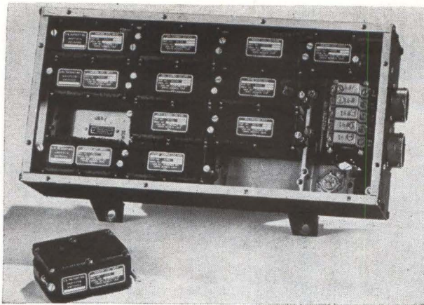
MODULAR control amplifier, built by Lear-Siegler, weighs 12½ lb and is 13 in. long
