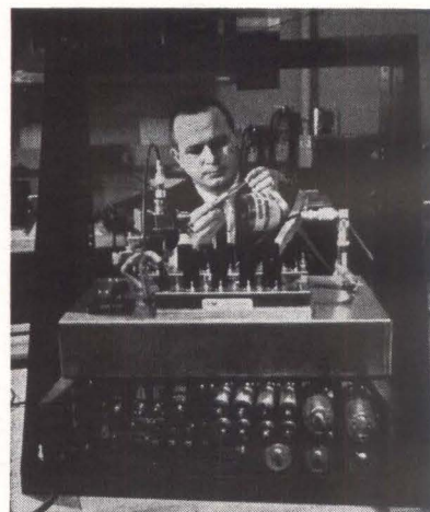
EXPERIMENTAL quartz demodulator for ruby laser is shown with inventor, Kenneth E. Niebuhr, of IBM Federal Systems Division
