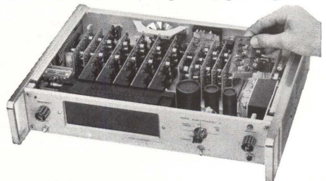
Note clean, compact, easy-to-service physical arrangement of new \Phi solid-state counters.
