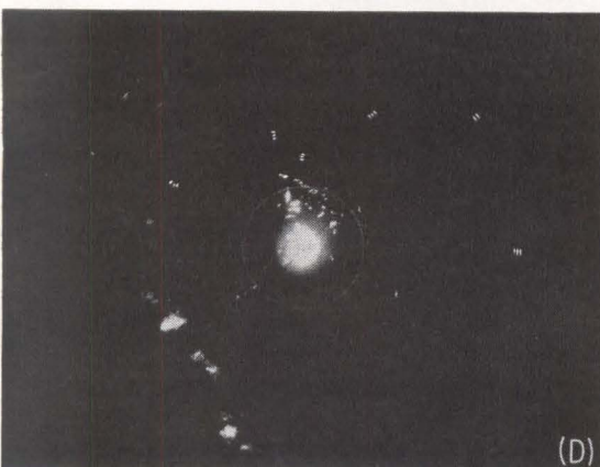
FIG. 1—Effect of some clutter-reducing techniques. Normal radar video (A); with circular polarization (B); using an mti receiver with circular polarization (C); and adding sensitivity time control (D)
