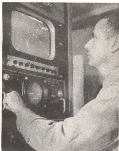
Under an experimental Coast Guard program, radar view of New York harbor is transmitted over uhf-tv channel 47. System uses a Raytheon storage tube which gives a persistent trace of moving ships. Craft in harbor equipped with tv set can determine their own position by maneuvering and watching their trace
