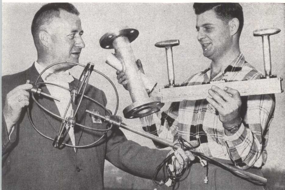
ACOUSTIC FLOWMETER developed by Westinghouse uses spherical array of acoustic probes to measure water currents in three dimensions. More conventional flowmeters are shown at right
