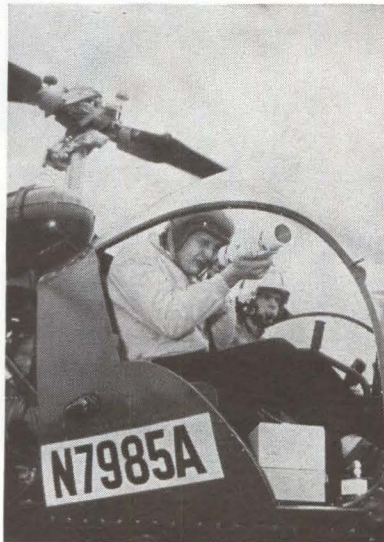
AIR-GROUND TV developed by Cubic Corp. and Cohu Electronics enables ground observers to monitor missile launches. Airborne portion consists of camera and transmitter each weighing about 5 pounds. Receiver has horizontal line resolution of 700 lines
