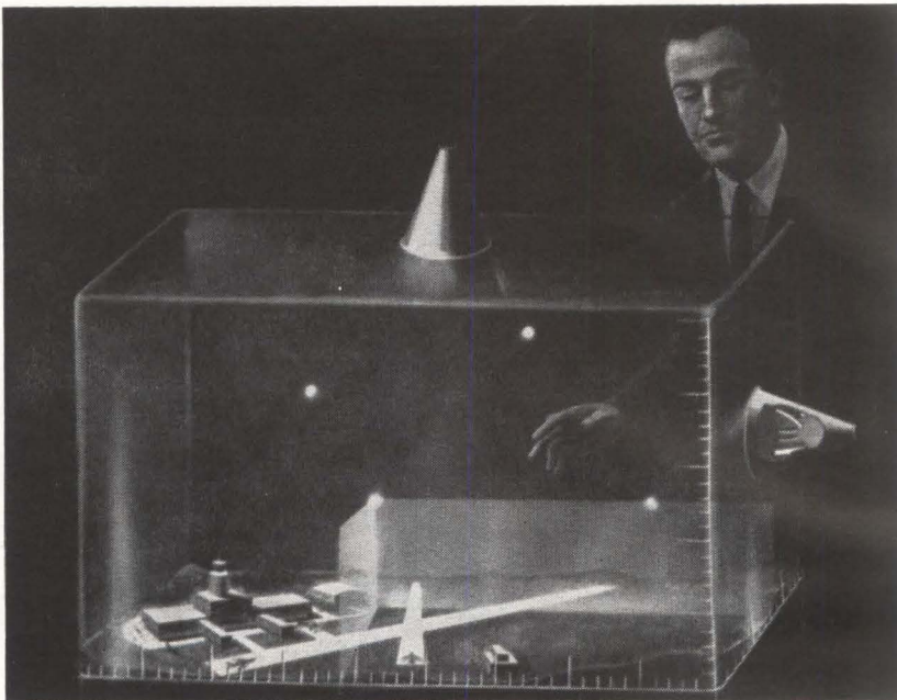
THREE-DIMENSIONAL DISPLAY using threshold excitation of mercury vapor, in artist's conception
