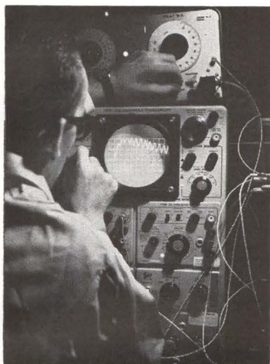
WAVEFORM carrying color information from retina of test animal to its brain is intercepted and analyzed on oscilloscope
