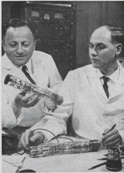
Electrostatic image orthicon was developed by General Electric Co. engineers Kurt Schlesinger, left, and Bernard Day. Reduced power, weight and size may now give it a place in military and space applications.
