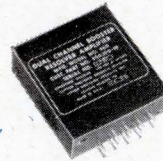
BOOSTER AMPLIFIERS, COMPONENTS OF THE NAVIGATION AND BOMBING COMPUTERS F-111 AIRCRAFT
