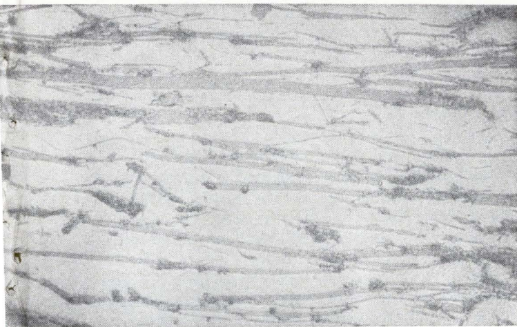
Layered structure of semiconducting glass-bonded mica, magnified 300X. Such high-strength composites can also be made with boron-nitride dielectric and graphite.
