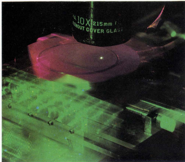
Many-circuited wafer is coated with photoresist, exposed in unique pattern by ultraviolet beam (bright spot).
