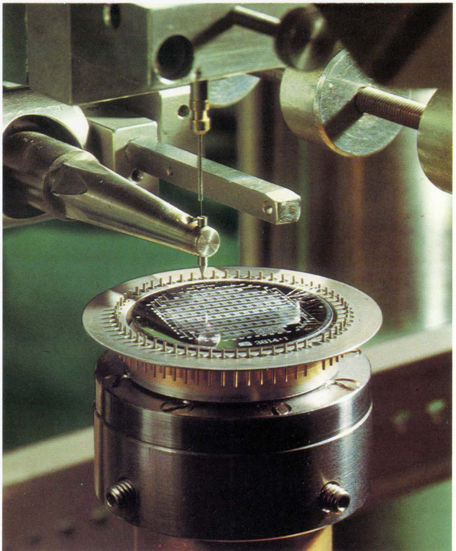
Blurred table is rapidly indexed to generate interconnection path under fixed beam.
