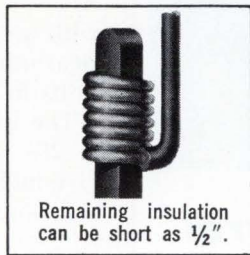
Wire is fully stripped, ready for wrapping tool.
