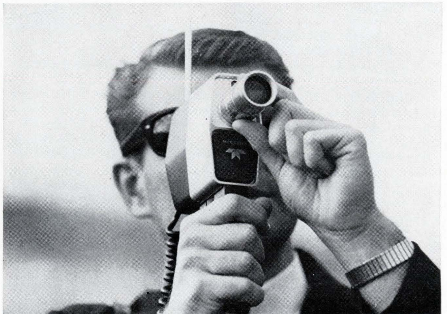
Commercial model of Teledyne's television camera-transmitter. Unit weighs 1½ pounds and will be introduced this year.
