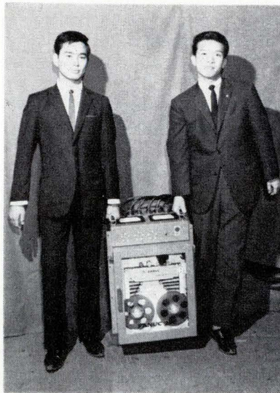
Lighter load. A switch to IC's for the logic circuits slashed the size and weight of Fujitsu's Fanuc 260 NC unit.
