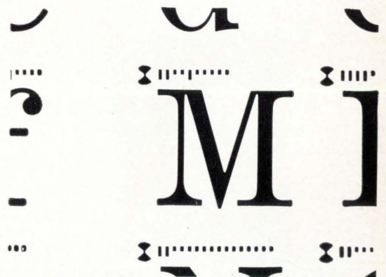
Servo system for horizontal axis control generates a position correction signal that locks the scan to the reference mark beneath the character. Reference and coding marks indicate how the character should be scanned and spaced.
