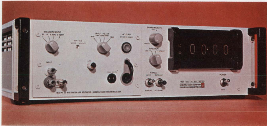
High or low. New dvm can measure quantities as small as a picoampere or a millivolt, and resistances as high as 50 megohms—with decibel readout.
