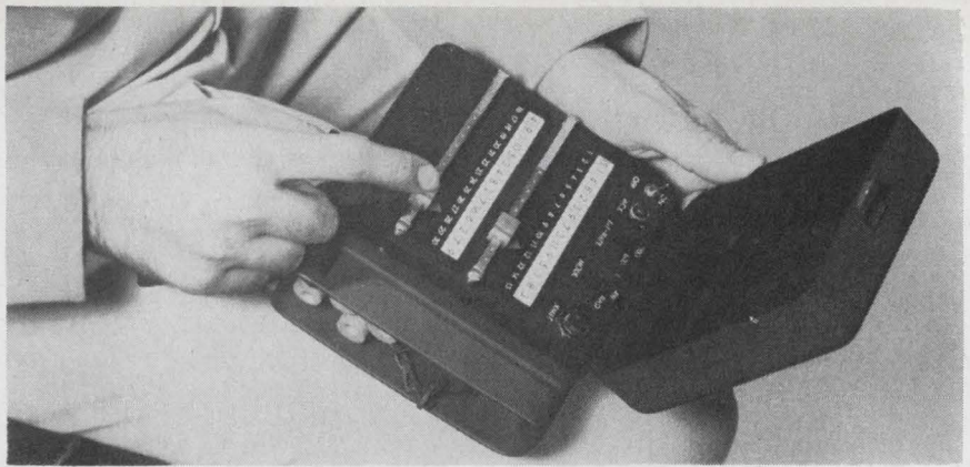
Out front. Forward observers use the fixed format message entry device to compose and store fire requests to battalion centers over radio links.
