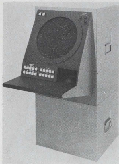
In the round. The tactical display backstops the digital plotter maps, used in the fire-direction centers, giving detailed data on small areas.
