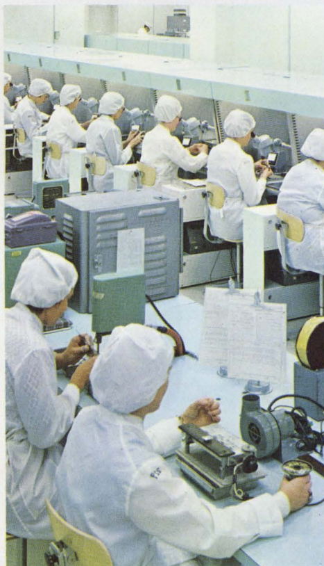
Partial view of clean room where HL relays are assembled, adjusted and sealed.
