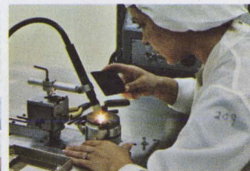
TIG (Tungsten inert gas) welding process is used to seal headers to cases.
