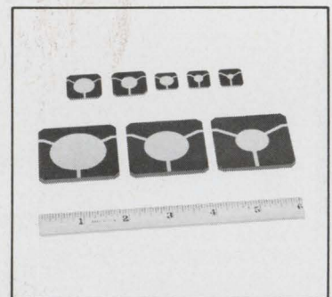
VARIOUS CIRCULATOR SIZES AND DESIGNS COVER 1.5 TO 13.0 GHz
