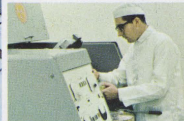
Hermetic seals of HL relays are verified with radio-active krypton 85.
