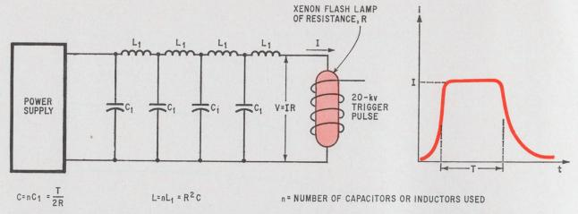
**Pulse-forming network.** This stores energy from the power supply and matches the lamp impedance to that supply. A trigger pulse ionizes the gas in the flash lamp and the stored energy discharges through the lamp.
