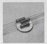
Multijunction rectifier called Ministac offers piv's of 3 kv to 7 kv. Average rectified current is 10 ma. Leakage current is 100 na. Leakage current is 100 na and maximum junction capacitance is 1 pf. Maximum recovery time is 100 nsec. Units measure 0.400 x 0.120 in. Units are metallurgically bonded at high temperature giving high strength. Semetch Corp., 652 Mitchell Rd., Newbury Park, Calif. [442]
