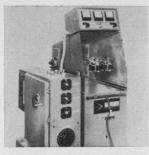
Coil encapsulator ACE-100 coats stator, transformer and other coils through a 3-step operation. After the operator places the parts on the tooling, hooks up the coils and presses the start button, the pre-heat, dip and post cure cycles are performed automatically. Windings are uniformly coated at 100 per hr. Possis Machine Corp., 825 Rhode Island Ave. So., Minneapolis. [425]
