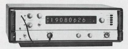
The 1191-Z is also available in a 100 MHz model that uses a 10-to-1 scaler. In all other respects performance is similar to that of its 500-MHz counterpart. Price is \$2040.
