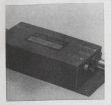
Solid state broadband amplifier model EBA1001 covers 10 to 400 Mhz. Noise figure is 8 db max; gain, 20 db minimum; gain flatness, ±0.5 db minimum; power output at 1 db gain compression, +20 dbm minimum; input vswr, 2.5 max.; output vswr, 2 max. The unit measures pulse, ECM, and RFI. E&M Laboratories, 7419 Greenbush Laboratories, N. Hollywood, Calif. [401]
