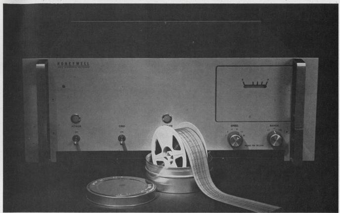
Easily installed, the new Microfilm Recorder Accessory makes high-quality archival records on inexpensive 35mm film.
