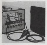
D-c differential voltmeter model 896A is a ruggedized unit that is waterproof, humidity proof, operates over a wide temeprature range and meets applicable military specs for shock and vibration. Range is 0 to 1,000 v in 4 ranges with 10% overranging. Accuracy is ±0.01% of input. Price is \$2,000. John Fluke Manufacturing Co., P.O. Box 7428, Seattle, Wash. 98133. [361]
