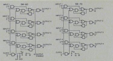
Fig. 1. Logic arrangement of SM-60 and SM-70 are similar except for output stage. The SM-70 reads out on clock pulse, while the SM-60 requires an "enable" pulse before giving an output.
