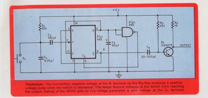
processes form the leading edge of the output pulse. After 100 nanoseconds,  $C_4$  will have discharged through  $R_2$  to a voltage that allows  $Q_1$  to return to saturation, and the falling edge of the pulse is formed.
