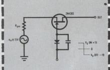
**SOLUTION:** Junction FETs are available in various ranges of  $V_{p}$  and  $r_{ds(on)}$ . This provides a trade-off between drive voltage and ON resistance. A good choice for this application is the 2N4393:
