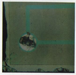
Advice from a vendor. The semicircular cracks at the lower edge of this chip are a rejection criterion suggested by an IC manufacturer during Raytheon's negotiations. They could give rise to loose particles of silicon during vibration or shock.
