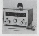
Internal linearizing bridges and digitizing circuits are employed in the series 8114 temperature indicators to provide direct, 4-digit display of inputs from platinum temperature sensors. Resolution of 0.01° is achieved, with temperature displayed in degrees C or F. Prices start at \$1,595. California Instruments Corp., 3511 Midway Drive, San Diego, Calif. 92110. [368]
