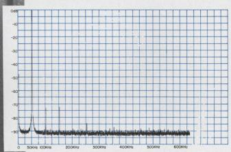
Signal with Line Frequency Related Sidebands-1 kHz signal with linerelated spurious FM-ing of fundamental using 10 Hz BW, 1 Hz/sec sweep rate.
