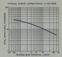
Fig. 1. Typical curve of capacitance versus reverse bias voltage for VVC diode (D6332A).
