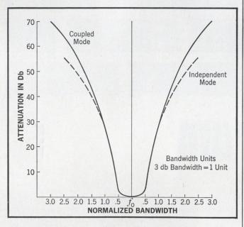
Go independent mode. Go coupled mode. You can go either mode with monolithic Clevite Uni-Wafer filters. They're smaller and more reliable (fewer interconnections) than conventional filters.
