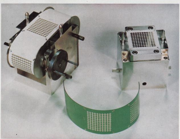
**Colorful amplifiers.** Red substrate contains array of 100 thin-film transistors; green substrate has 658. Both types of masks are positioned between pins of the supply spool, which is placed in a vacuum chamber.
