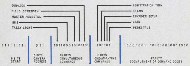
Command code organization. The basic command word, not including the nine-bit start signal, is made up of 24 bits. After each word is transmitted, it is repeated with 1's and 0's interchanged to detect any false information.
