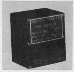
Analog-to-digital encoder model 1250, displacing only 6 cu ln., can encode ±10 v input into 12 binary bits of data at the rate of 1 µsec per bit. Successive approximation measurement is used to provide a resolution of one part in 4,096 with an accuracy of ±0.05% in ambients ranging from 0° to 50°C. Phoenix Data Inc., 3065 W. Fairmount Ave., Phoenix. 02154. [387]
