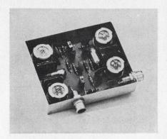
Listener. The receiver picks up the 100-khz signals sent by loran stations.
