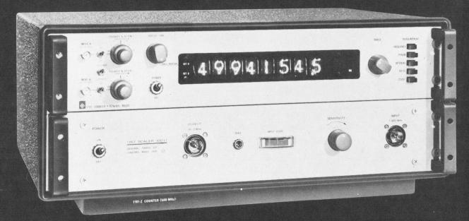
GR's new 1191-Z Counter is a 500-MHz general-purpose counter that has full counter-timer functions, programmability, high-speed data access, eight-digit readout, and a high-precision time base . . . and it costs only \$2190!
