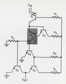
Self-defense. Extra transistor, Q3, and the configuration of Q4, Q5, and Q6 shield against false triggering.
