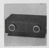
Miniature, 50-ohm rotary attenuators in the 500 series are for lab and accessory use. Model 550 covers 0 to 110 db in 1 db steps; model 570 covers 0 to 80 db in 1 db steps; model 560 covers 0 to 11 db in 0.1 db steps. They feature low vswr and flat frequency response from d-c to 2 Ghz. Prices range from \$225 to \$275. Texscan Corp., 2446 N. Shadeland Ave., Indianapolis. [403]
