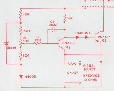
Electronic time delay circuit
