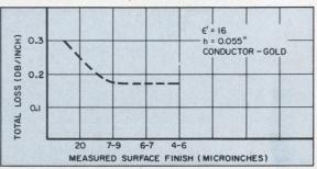
TOTAL LOSS - VS - SURFACE FINISH OF SUBSTRATE
