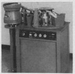
Sorter type 802 automatically inspects and sorts disk varistors and other disk components. It provides test rates to 7,200/hr. High yield is produced by accurate measurement achieved with 4-terminal (Kelvin) probe. Two separate terminals make contact with each side of disk. Contact resistance is below 50 milliohms. Daymarc Corp., 40 Bear Hill Rd., Waltham, Mass. [424]
