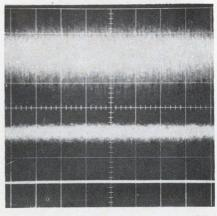
. . . and out. These are results when noise goes through twisted pair, standard busbar, or new busbar.
