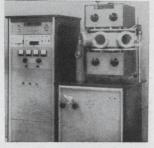
Sputter etching system 8550 for thin film products uses r-f plasma-produced ions. As substrates move through the chamber, they can be cleaned by etching, coated with a resistor material such as tantalum, and then the resistor coating can be trimmed by etching. Price for basic system is \$12,900; delivery, 4 to 6 weeks. Materials Research Corp., Orangeburg, N.Y. 10962. [428]
