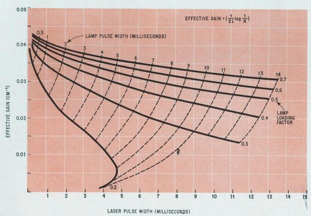
Reflectance. If the lamp loading factor and either the lamp's or laser's pulse width is known, this chart can be used to find the necessary effective gain. The length of the ruby rod is then substituted in the effective-gain equation to give the reflector requirements.
