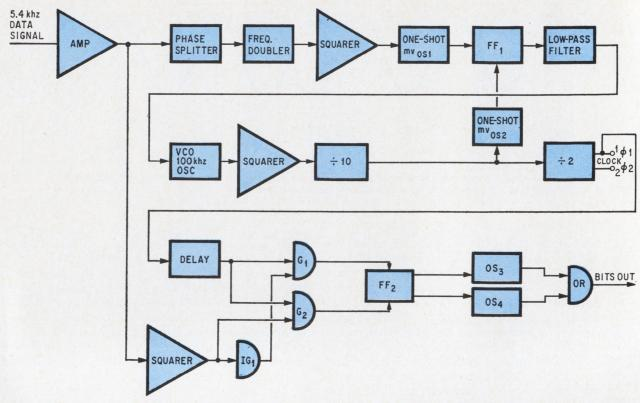
Bit decoder. The incoming coded signal from the base station is decoded by a series of operations, including frequency multiplication and division. The detected output bits are then used to switch circuits or vary controls.
