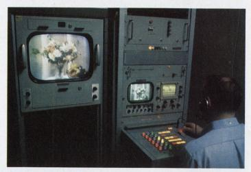
On base. Station is functionally equivalent to a conventional studio control console.
