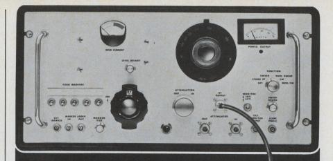
You don't need a sweep generator to run a high intensity lamp, but the 8-watt output of Telonic's new PD series sweep generators will allow you to test varactor multipliers, align high-power transmitter and amplifier chains, establish multi-test station swept signal distribution systems, and test high-loss and non-linear devices—among other things.
