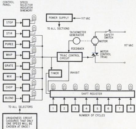
**Kitchen aid.** Food blender, designed with Motorola integrated circuits, will soon be made available by John Oster Manufacturing. The design eliminates push buttons and switches. Speed selection is made by touching insulated capacitance plates.
