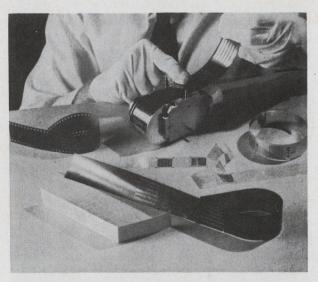
Continuous. Without breaking the vacuum, transistors can be made on a variety of substrates wound on spools.
