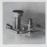
Silicon PIN switching diodes of the series 47000 is represented by the 47004, which has a peak power of 15 kw with switching speed of less than 500 nanoseconds. Minimum breakdown voltage is 500 v. Units are suited for control applications including r-f switching, limiting, duplexing and phase shifting. Microwave Associates Inc., Burlington, Mass. [440]
