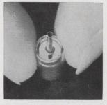
A sapphire-insulated vacuum feedthrough limits vacuum leakage to less than 10-10 cc of helium per sec. The device, designed for the conductance of minute electrical currents between the atmosphere and vacuum-enclosed circuits, is expected to have wide application in the electronics and spectrometry fields. Cary Instruments, 2724 S. Peck Rd., Monrovia, Calif. [344]
