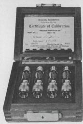
Attenutor Sets are used world-wide as standards in labs and on production lines. Attenuator Sets include 4 or 8 specially selected and calibrated (at 1 GHz intervals) 3, 6, 10, and 20 dB Precision Fixed Coaxial Attenuators. They are handsomely packaged with their individual laminated calibration data in a custom made walnut storage case.
