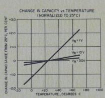
Fig. 2. Change in capacitance with temperature normalized to 25°C (D6332A).
