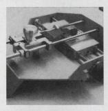
Ceramic/glass substrate scriber Is useful for producers of hybrid circuits to scribe material Into any rectangular size required. Work is inserted into a holding chuck and the operator makes a visual alignment by indexing the driving lead screw until scribe path coincides with diamond scribe. Price, \$590. Mechanization Associates, 2622 Frontage Rd., Mtn. View Calif. [422]
