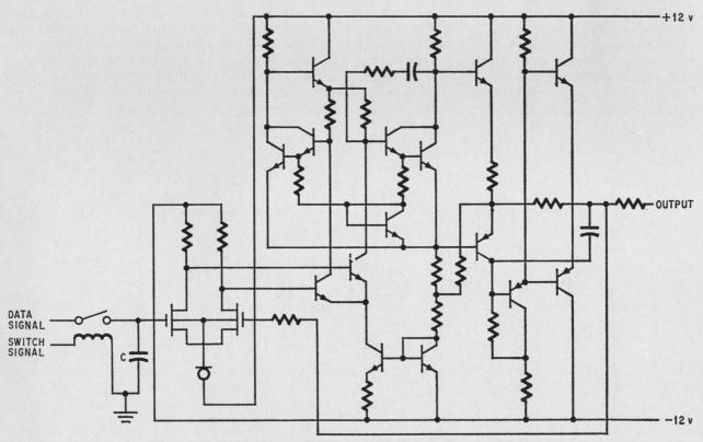
Sample hold circuit. Solid state equivalent of motor-driven potentiometer uses low-leakage polycarbonate dielectric capacitor with high-impedance MOS FET differential amplifier and IC op amp to achieve memory capability.
