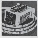
Solid state time delay relay TDR2 is for industrial and commercial use in driving solenoids, relays, small motors and similar loads. With a repeat accuracy of 3%, timing ranges available are 0.1-10, 0.3-30, 0.6-60, 1.2-120, 1.8-180 sec, over a temperature range of 0° to +55°C. Maximum timing variation due to temperature is ±4%. Tansitor Electronics Inc., Bennington, Vt. [345]
