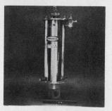
Gallium arsenide semiconductor laser model RSL-5 provides 4 w of c-w output power. It consists of a liquid helium dewar and a demountable semiconductor laser header. Output of the unit is at 8,400 angstroms and operating temperature is 4.2°K. Price is \$12,390 or \$4,245 without dewar with 60 day delivery. Raytheon Co., Foundry Ave., Waltham, Mass. 02154. [388]
