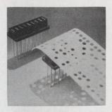
Plastic phototransistor array FPA-700, for reading standard 8-channel punched paper tapes, consists of 9 NPN phototransistors in an 18-lead package designed for ease in handling and mounting. It operates at a temperature range of -40°C to +85°C. Price is \$21 each in quantities up to 99. Fairchild Semiconductor, 313 Fairchild Drive, Mountain View, Calif. [437]
