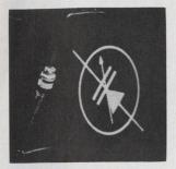
Voltage variable capacitance diodes in the IN 5139-39A through IN5148-48A series provide Q's ranging from 200 to 350 at -4 v d-c, tuning ratios from 2.7 to 3.4, and center capacitance values from 6.1 to 51.7 pf. Maximum working voltage rating is 60 v d-c. Units are for uses such as voltage tuned filters. Crystalonics, A Teledyne Co., 147 Sherman St., Cambridge, Mass. [436]
