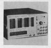
Digital data simulator 912 (7½ in. high by 13½ in. wide) programs 960 bits of binary information at the front panel using 320 tiny octal-weighted programing pins. The 960 serial bits can be clocked out at rates to 10 Mhz. In the parallel mode, up to eighty 12 bit parallel words can be outputed at rates up to 5 Mhz. Moxon Electronics, 2309 Pontius Ave., Los Angeles. [385]
