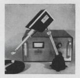
Existing solder pot conversion to ultrasonic tinning is made possible by an add-on unit designed for all component lead tinning applications. Ultrasonic tinning results in cost savings by eliminating fluxing and cleaning steps, and improving shelf life and serviceability. The unit may be used with any type solder. The Redford Corp., 968 Albany-Shaker Road, Latham, N.Y. 12110. [426]
