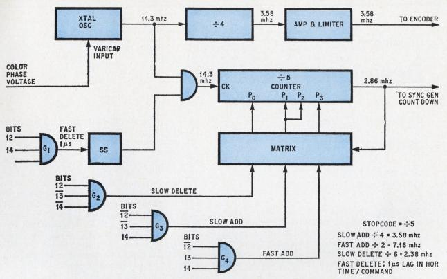
Horizontal sync and color phase. Sync is controlled by varying the division of the counter; the color subcarrier is varied in frequency and phase by using a varicap to pull the master clock oscillator.
