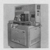
Automatic dicer Mark III dices one silicone, germanium, or titanate wafer every 80 seconds. Depending upon chip size, it can turn out more than 4,000 transistors, diodes, capacitors, or IC's in a little more than a minute. The dicing is accomplished by 0.002 in. cutting disks, precision spindle, and slurry bombardment. Taft-Pierce Mfg. Co., Mechanic Ave., Woonsocket, R.I. [423]
