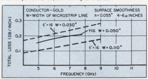
TOTAL LOSS — VS — FREQUENCY FOR VARIOUS STRIP WIDTHS
