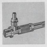
Universal r-f precision tunable probe model 229C is compatible with all coaxial and waveguide slotted lines with 3/4 in. diameter standard mounting holes. It is tunable throughout the entire range of 0.90 to 18.0 Ghz. The r-f output from the probe enables it to be used with microwave receivers or other external detectors. Narda Microwave Corp., Commercial St., Plainview, N.Y. [405]
