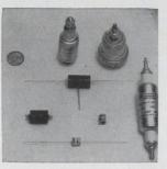
Precision spark gaps types 2009-01 through 2009-04 have voltage breakdown capability from 450 v to 1,500 v. All feature ultrafast response and insulation resistance of greater than 1,000 megohms. Maximum surge current handling capability of the line ranges from 10,000 to 40,000 amps on a 10 x 20 µsec waveshape. Joslyn Electronic Systems, 6868 Cortona Drive, Goleta, Calif. [347]
