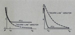
Fig. 1. Capacitance and resistance versus bias voltage for PTV diode and normal abrupt-junction varactor.
