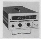
Frequency counter model 7015 is for portable use in the communications field. It has a direct counting range of 100 Mhz, while built-in automatic prescaler extends the upper range from 100 to 500 Mhz, thus providing continuous coverage into the uhi region. Net weight of the unit is 13 lbs. Price is \$1,975. Systron-Donner Corp., 888 Galindo St., Concord, Calif. 94520. [363]
