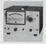
Solid state picoammeter 410A can be used for measuring and amplifying signals as low as 3 x  $10^{-14}$  amp from ion gages, liquid-level gages, gas chromatographs, thickness gages, phototubes and mass spectrometers. On the  $10^{-8}$  to  $10^{-12}$  ampere ranges, zero drift with time is less than 0.5% of full scale per wk. Keithley Instruments Inc., 28775 Aurora Rd., Cleveland. [366]
