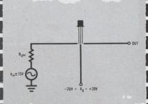
REQUIRED: Select FET to switch ±15 V signals . . . maximum available drive voltage is ±20 V. Use either a MOS or a junction type.
