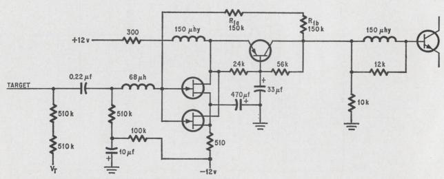
Camera-tube preamplifier. Featuring parallel field effect transistors, circuit stabilizes low-frequency gain with respect to temperature with a low-capacity, 40-decibel-gain feedback loop.
