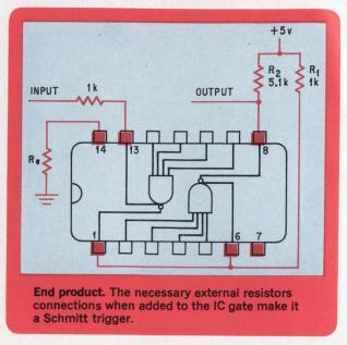
input signal increases to the input threshold,  $Q_1$  turns on. The input threshold is determined by the two offset diodes, the base-emitter junction of  $Q_1$ , and voltage drop across  $R_e$  due to the emitter current of  $Q_2$ . With  $Q_1$  on,  $Q_2$  turns off and the output goes high. When the input signal drops to a level again determined by the diodes and the  $IR_e$  drop,
