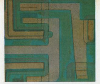
Notched. A defect in the metalization mask created this notch in the metalization. If it extended more than halfway across the metalized path, it would be cause for rejection.
