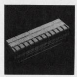
Thirteen-track flying magnetic head for disk memories provides reliable performance at packing densities up to 1,300 bits per inch. Track width is 0.015 in. spaced on 0.125 in. centers. Inductance is 40  $\mu h$  per winding leg and gap length is 200  $\mu$  in. Prices start at \$380 and vary with quantity. Applied Magnetics Corp., 75 Robin Hill Rd., Goleta, Calif. [383]
