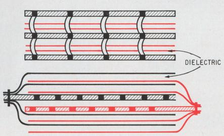
The reason why. Most laminated busbars are stacks of thick, metal plates. But a busbar's conductor area, hence its capacitance, is more when the conductors are thin strips of metal that are interlocked like fingers on folded hands.
