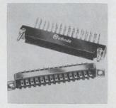
Two-part fork contact p-c connectors are designed to permit tying-in printed circuits directly to the unit's cabling. Features of the new series, available with either 31 or 41 contacts, include glass-filled diallyl phthalate Insulators, coated aluminum shells on the male connectors, and solder type terminals for wiring. Methode Electronics Inc., W. Wilson Ave., Chicago. [348]
