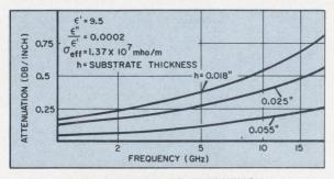
ATTENUATION VS FREQUENCY FOR 50 OHM MICROSTRIP LINE ON VARIOUS SUBSTRATE THICKNESSES Similar progress has been made in the understanding and control of substrate microstructure, surface finishing, ground plane spacing, strip width, conductor dimensional tolerances and impedance matching for minimum losses in microstrip transmission lines.
