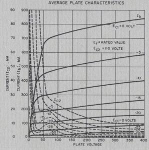
Peak plate current vs peak screen-grid current. Note low knee voltage at various bias ratings. At a plate voltage of 60 volts with zero bias, peak plate current is 700 mA and screen-grid current is 32 mA,  $\frac{\text{ib}}{\text{ic2}}$  ratio is better than 20 to 1.
