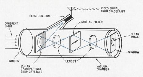
**Optical filter.** The signal (crescent) buried in the noise (vertical bars) is recovered by inserting a filter in the plane of the two-dimensional Fourier transform established by the first lens. The filter removes the noise transform; a second lens reconstructs the image from the signal transform.
