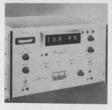
Direct reading 1-Mhz capacitance tester model 1206 features IC's for fast test time of 50 msec. It also has a 50% overrange which minimizes switching at often used test values, permitting faster testing. The unit provides direct digital readout of measurements to 0.001 pf and accuracies of  $\pm 1/4\%$  of reading. Micro Instrument Co., 12901 Crenshaw Blvd., Hawthorne, Calif. [365]
