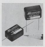
Fixed time delays ranging from 0.1 to 15 sec with accuracies of ±5% and ±10% are offered by a line of solid state time delay relays. Units have an output rating of 0.7 amp and a size volume of no more than 0.25 cu in. Weight is 0.5 oz. Input voltage range is 14 to 35 v d-c. Minimum holding current is 10 ma. ADC Elecronics Corp., 1227 W. 254 St., Harbor City, Calif. [346]
