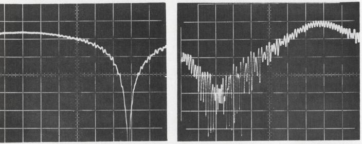
Losses. Insertion loss, left, is greater than 35 decibels at 3.56 Ghz, indicating a fault. Return loss, right, is 11 db.
