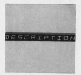
Custom-produced 16-segment bartype readouts can display over 65,000 discrete patterns including a complete alphanumeric presentation, digraphs, and conventional symbols. Illumination for segments making up each character is supplied by light generated by lamp blocks. Tung-Sol Div. Wagner Electric Corp., 1 Summer Ave., Newark, N.J. 07104. [384]
