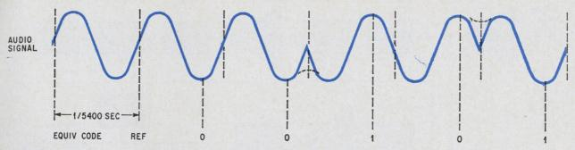
**Encoding control signal.** Information is encoded by phase shifting a 5.4 kilohertz subcarrier 180° to denote a binary 1. The absence of a phase shift on successive cycles denotes binary 0.
