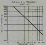
Fig. 3. Normalized Q of VVC diodes over frequency range.
