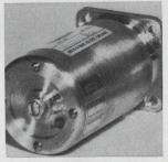
X-band solid state power generator E3288 is a low noise, electronically tuned device suited for local oscillator or test source use in commercial and military applications. Operating frequency is 8 to 11 Ghz with a tuning range of 400 Mhz. Power output is 10 mw. The unit operates from a -17.5 v stabilized supply. The M-O Valve Co. Ltd., Brook Green Works, London W.6. [408]
