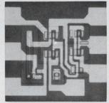
Model LM703 is a monolithic r-f/i-f amplifier. The circuit has a low internal feedback which guarantees a high stability-limited gain. Features include a forward transadmittance of 35 mmhos, input conductance of 0.03 mmho, output conductance of 0.02 mmho, and peak to peak output of 4 ma. National Semiconductor Corp., 2950 San Ysidro Way, Santa Clara, Calif. 95051. [443]
