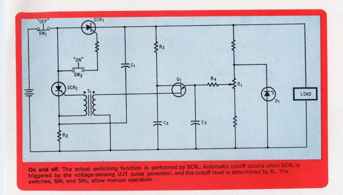
If visual indication of cutoff is desired and if a small continuing drain on the battery can be tolerated, R<sub>1</sub> can be replaced by a low-current incandes-
