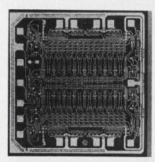
Unforgetting. The XC170 is a 128-bit read-only memory, compatible with DTL and TTL.
