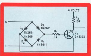
Selection. Switching takes place in the transistor only when a signal is present at either the A or B input—never both.
