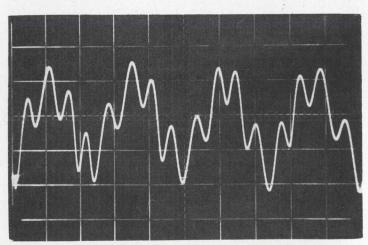
Good and bad. Display from 32-foot 4-inch length of open RG-58 U coaxial cable indicates, with 2-feet per ripple calibration, that cable is 32 feet 6 inches long, left. Accuracy is typically better than 5%. The display is affected if the cable is crimped 8 feet from the measurement end, right. The pattern has two parts: 16+ ripples superimposed on a four-ripple pattern caused by the crimp and indicating a fault at the 8-foot point.
