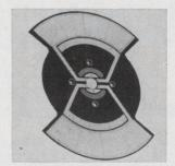
A Schottky barrier unit has an array of 8 circular segmented photodiodes on a 3-in. diameter circuit board. The photoexcited carrier transit time is 10-9 sec and capacity per unit area is 100 pf/cm². The unit is designed for use as an automatic shutter control on a high speed military camera. United Detector Technology, 1728 21st St., Santa Monica, Calif. [439]
