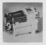
Medium duty relay JBJA offers small size, long life, and reliability. Standard silver contacts will switch 10 amps current for a minimum 250,000 operations or 4 amps for 2 million operations. They also possess a switched voltage rating of 380v a-c max. or 200 v d-c max. Typical operating times are from 4 to 7 msec. ITT Jennings Div. of ITT Corp., Box 1278, San Jose, Calif. [342]
