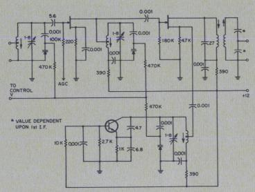
FM tuner uses VVC diodes for tuning with FETs in the RF and mixer stages. For optimum performance across the entire FM band, the tuning diodes should be matched within 10% at the nominal rated voltage.
