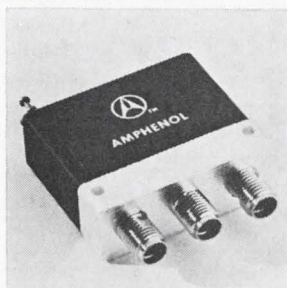
Miniature coaxial switch features high isolation over its entire zero to 12.4 Ghz operating range. The spdt units provide 60 db minimum of isolation at 12.4 Ghz. Vswr at this frequency is 1.5 and insertion loss is 0.5 db maximum. Units are rated at 50 w of r-f power with an operating time of 15 msec. Amphenol RF Division, Bunker-Ramo Corp., E. Franklin St., Danbury, Conn. [407]
