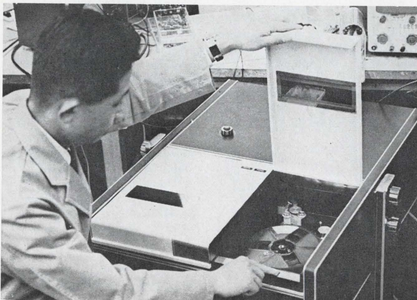
Fast whirl. Matsushita video tape copying equipment can duplicate a 2,400-foot reel of master tape in just two minutes. Bifilar winding of master and slave tapes on the same reel is what makes machine a speedster.
