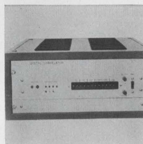
On-line digital correlator DC-100 is suited for filter functions with any data gathering or pulse recognition equipment, such as receiving systems or recorders used in radar, sonar, and other echosounding applications. Data storage is 3,072 8-bit words per channel, 12.28 sec at 4 msec rate. Price ranges from $20,000 to $22,000. Mandrel Industries Inc., Box 36306, Houston. [404]
