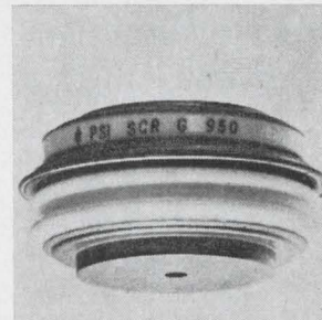
MegaPack scr is being used in a-c and d-c motor speed controls, solid state contactors and electro-mechanical power supplies. When mounted in a 3-phase full wave bridge, it can control up to 1 Mw at 900 v d-c, without the cost or complexity of paralleling. It is available in ratings of 650, 850 and 950 amps rms. Power Semiconductors Inc., 90 Munson St., Devon, Conn. 06460. [442]
