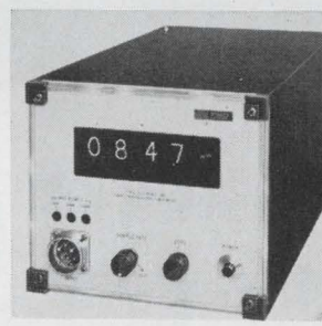
Digital thermoelectric power meter D6685 is designed to provide an accurate readout of average power of c-w, pulse, a-m or f-m signals. It offers power ranges corresponding to 0.03 \mu w to 100 mw and -45 dbm to +25 dbm. Accuracy is provided by a solid state d-c amplifier that includes 100 db of feedback. PRD Electronics Inc., 1200 Prospect Ave., Westbury, N.Y. 11590. [363]
