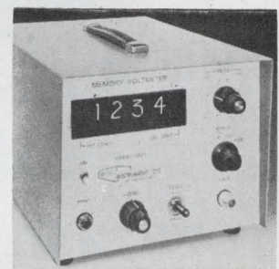
Memory voltmeter 5203, featuring a digital readout of d-c to 50 nsec pulses and amplitudes to \pm 1,000 v in 4 ranges, providing 100% over-ranges and BCD output, comes in a half-rack dual shielded cabinet. It will measure and hold the peak amplitude of one-shot or transient pulses, as well as repetitive pulses. Micro Instrument Co., 12901 Crenshaw Blvd., Hawthorne, Calif. [364]
