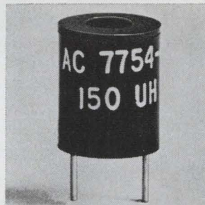
High Q miniature variable inductors AC7754 are offered in nominal inductances ranging from 0.1 \mu h to 4,700 \mu h. Designed for p-c application, the units measure 13/32 x 1/2 in. Two mounting terminals are spaced 9/32 in. on center for vertical mount. Tuning access is from either end. Approximate price is $1.50 in quantities. Automatic Coil Co., 76 E. 2nd St., Mineola, N.Y. [343]
