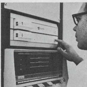
Cartridge-loaded system called Cartri-File provides PDP-8 computers with 4 digital tape transports. The system can be used to sort, match, collate and merge data. The tapes also provide program loading, off-line storage for memory dumps, and buffering for uninterrupted data accumulation. Price is $5,700. Tri-Data, 800 Maude Ave., Mountain View, Calif. 94040. [401]
