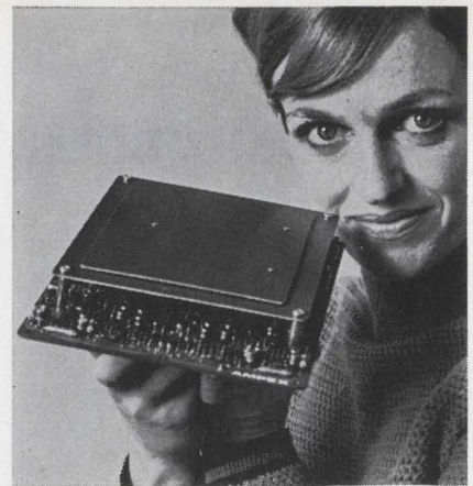
Minimem. Core storage unit is suited for jobs in displays and terminals.
