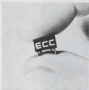
Metalized polyester Flat-Pak capacitors offer a low profile unit 0.225 in. high. Package width of all units is 0.385 with lead break-out at 0.300 center-to-center. Length varies from 0.100 for the 0.001 \mu f unit to 0.900 for the 1 \mu f unit. Capacitors come in more than 100 standard values rated at 50 v. Engineered Components Co., 2134 W. Rosecrans Ave., Gardena, Calif. [342]
