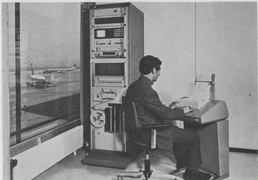
Monitoring noise. At Stuttgart's civil airport, this automatic system samples aircraft noise, prints out details every time pre-set levels are exceeded. Teletype is used to alert authorities to high noise events.
