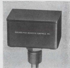
Mercury thermostats can be fixed set at any temperature between -20° and 200° F. Once calibrated, the unit will maintain the temperature to within 0.05° C over one year or 100,000 operations. It switches 2 amps a-c or d-c and comes with a plastic control housing and an aluminum or stainless steel probe. Philadelphia Scientific Controls Inc., 1135 Cedar Ave., Croydon, Pa. [345]
