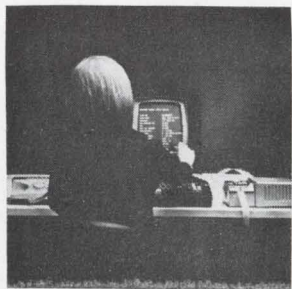
Noiseless, high-speed display/tape system series 5700 eliminates separate verification and enables ordinary typists to prepare error-free paper tapes. It features a television-like screen which displays an exact replica of a source document and provides visual verification of all typed data before it is punched on tape. Sanders Associates Inc., Nashua, N.H. 03060. [426]
