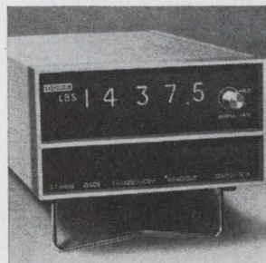
Digital weight readout DS-100-T2 provides readout directly in pounds, kilograms, or other engineering units when connected to strain gage load cells. It contains digital transducer conditioning including bridge excitation, balance and span, and millivolt per volt ratiometric measurement and readout circuitry. Doric Scientific Corp., 7969 Engineer Rd., San Diego, Calif. 92111. [365]
