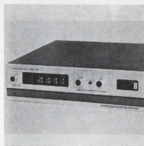
Digital pyrometer eliminates conformity errors with a multiple track scanning disk that is read optically. Units cover 3 temperature ranges—300° to +700°F, 0 to 1400°F and 0 to 2400°F—in standard models. The pyrometer consists of a basic readout module, designated DPM740, and a plug-in thermocouple sensor adapter. Consolidated Ohmic Devices Inc., Carle Place, N.Y. [363]
