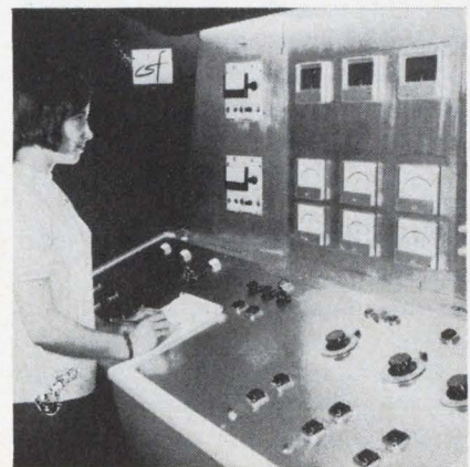
Plantation punch. Like an atom-smasher, Thomson-CSF's new machine accelerates particles for bombardment of a target, in this case semiconductor wafers. Simple controls allow in-plant use.
