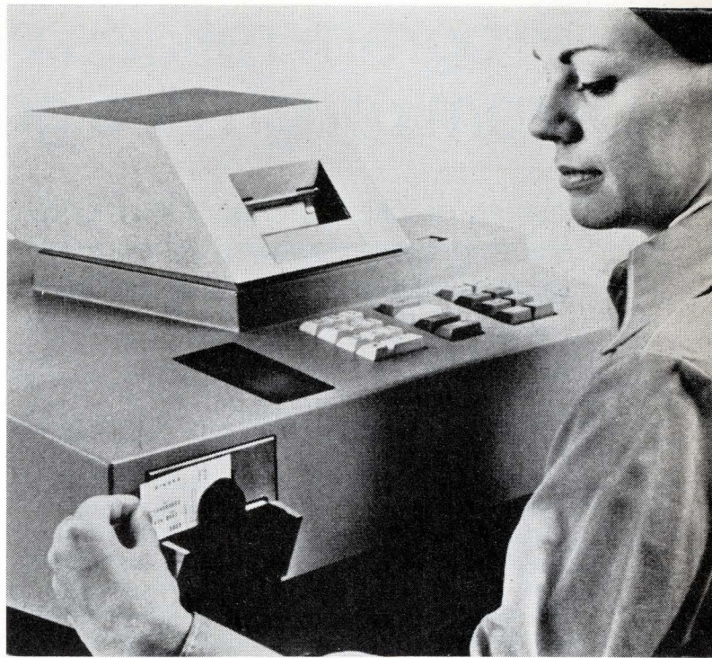
6. Things Italiano. The Olivetti TC 601 terminal, shown here, reads magnetic code merchandise tags. Terminal is part of storewide inventory control and sales data collection system controlled by minicomputer. It can also be used as a stand-alone register.
