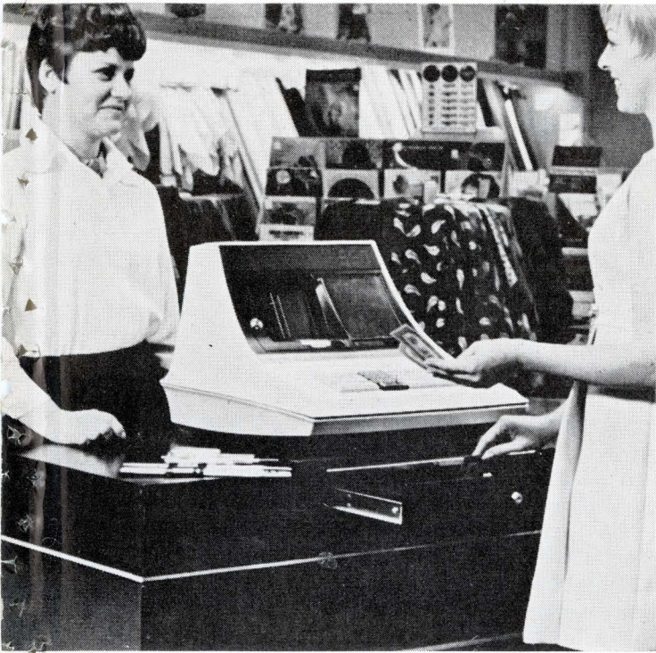
5. Store's store. Friden's Modular Data Transmission System (MDTS) terminal uses a continuous tape loop in a $650 module for daily transactions to the data processing center for updating inventory, recording charge purchases, and initiating reorders.
