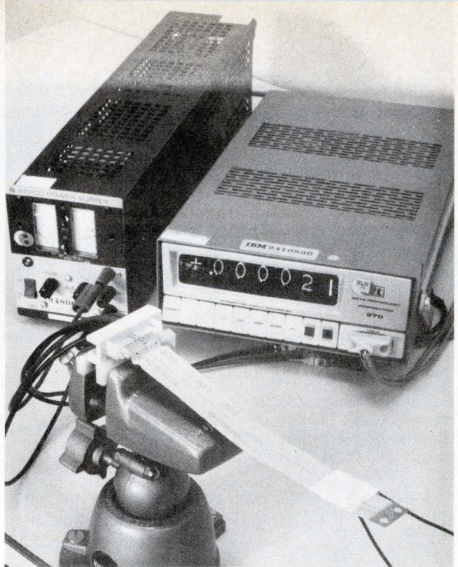
1. Test arrangement. Measurement tests joint between bus and connector. Soldered assembly, in jig, is shown close up in Fig. 4.
