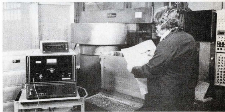
3a. Voice-created tape. Operator creates NC tape for Hillyer milling/drilling machine by speaking machining instructions into microphone. At left is the speech-recognition preprocessor-minicomputer unit, topped by an alphanumeric display that flashes each voice command for verification and also displays the next entry required.
