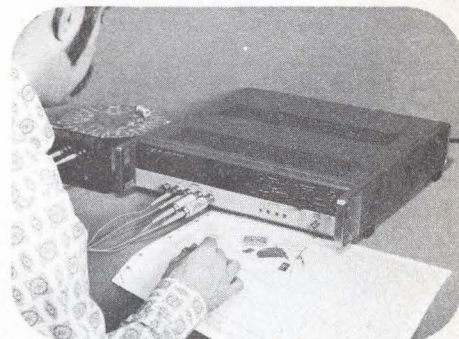
Typical uses for the 4271A LCR meter include: testing discrete components and varicap diodes, checking semiconductors, and L or C examinations of delay lines.
