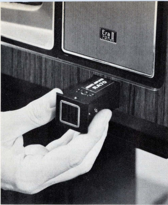
3. Plug-in remote. Admiral's optional remote-control system can be installed by the user on any five new models with the built-in adapter. The set owner removes a cover plate and plugs in the remote-control amplifier. Amplifier and hand-held unit retail for $99.95.
