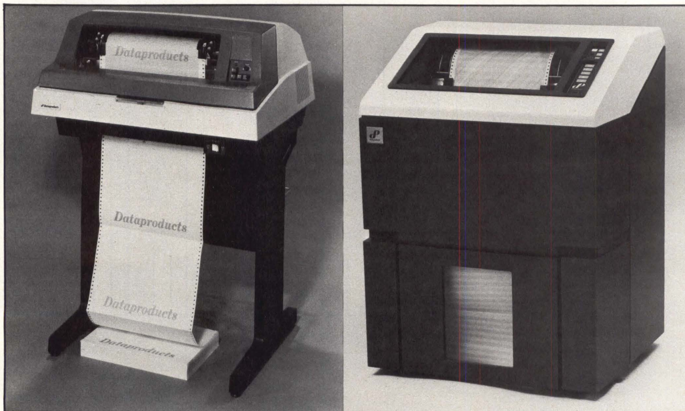
Fig. 3. Two band printers from Dataproducts Corp. illustrate the adaptability of band mechanisms. The 300-lpm model B-300 (left) is a pedestal-mounted printer priced at less than $4000 in 100-unit OEM quantities. The 1500-lpm model B-1500 (right) is a floor-standing model with a 60-dBa acoustic cabinet that sells for $11,300 in 50-unit OEM quantities. Both printers print 132-column, six-part forms and are available with 12-channel tape-controlled or direct-access vertical forms units. More than 250 bands in 50 font styles are available for B series printers.
