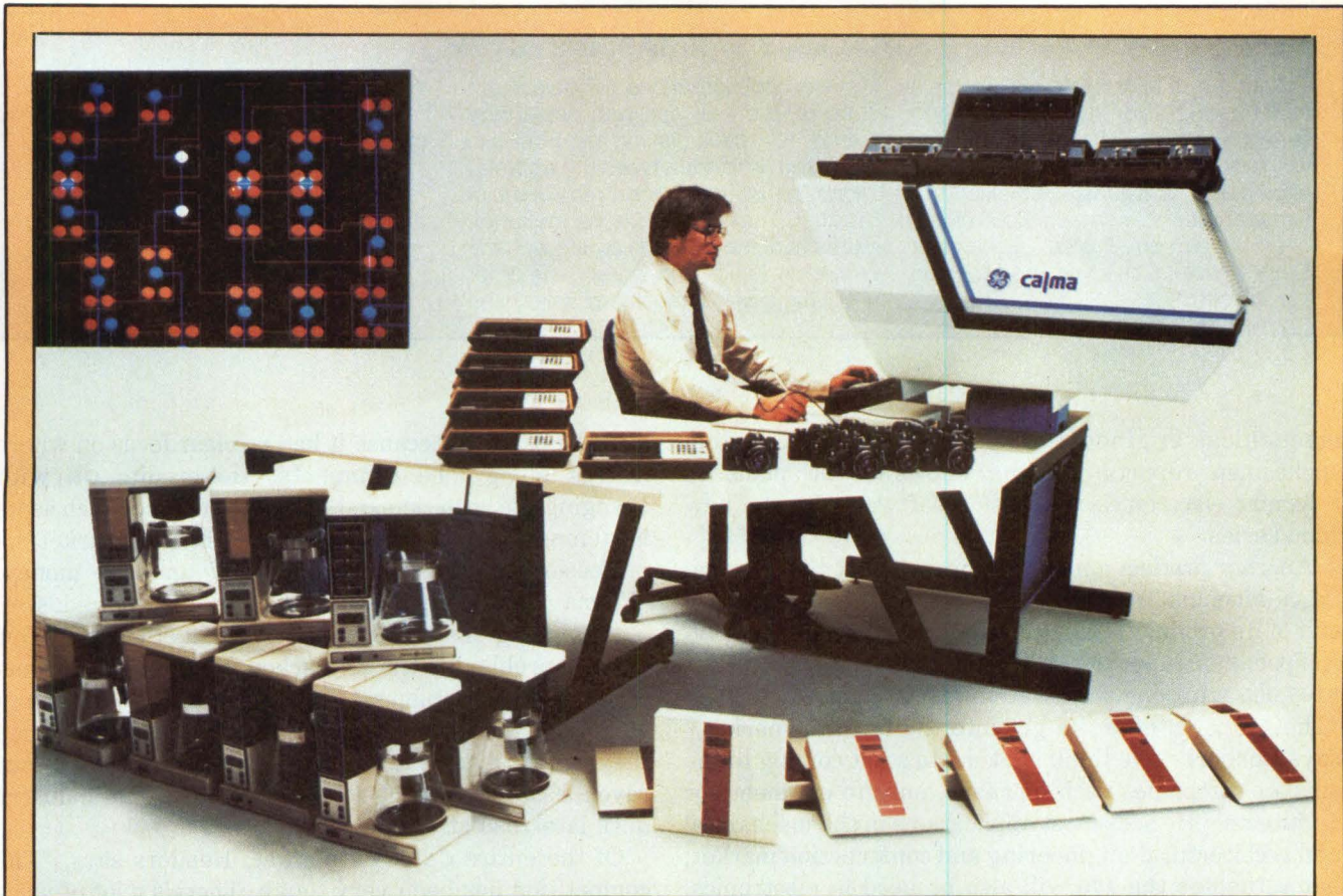
Screen shows a symbolic drawing of circuit elements used in VLSI design. The display is created by using STICKS, Calma's symbolic IC-design system.
