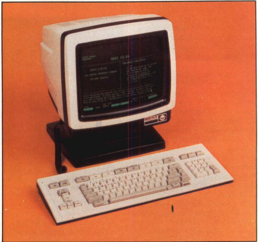
Beehive International's ATL-008 terminal's ergonomic design features a detached keyboard with 14-station numeric keypad with Enter key.
