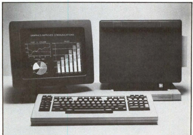
IWS-110 and IWS-120 graphics workstations from Convergent Technologies feature bit-map graphics in vector or raster mode. The workstations are hardware- and software-compatible with previous workstations in the series.
