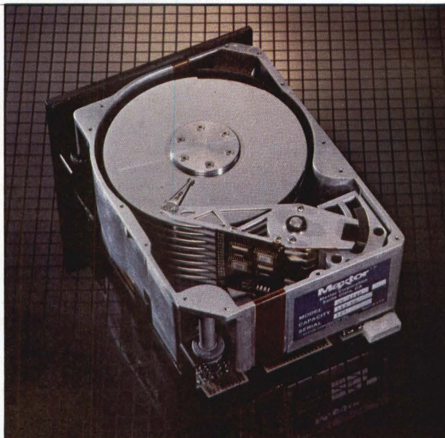
Maxtor XT-1000, 5¼-in. Winchester disk drives provide as much as 140M bytes of unformatted storage on eight plated disks with an average access time of 30 msec.
