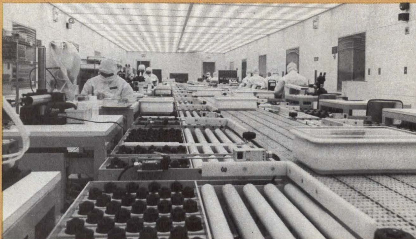
Class 100 clean tunnel assembly line produces Shugart 5¼-in. rigid disk drives. Automated conveyor system provides single-direction movement of the drive from unassembled components to final testing. Each tunnel can produce 100,000 drives per year.
