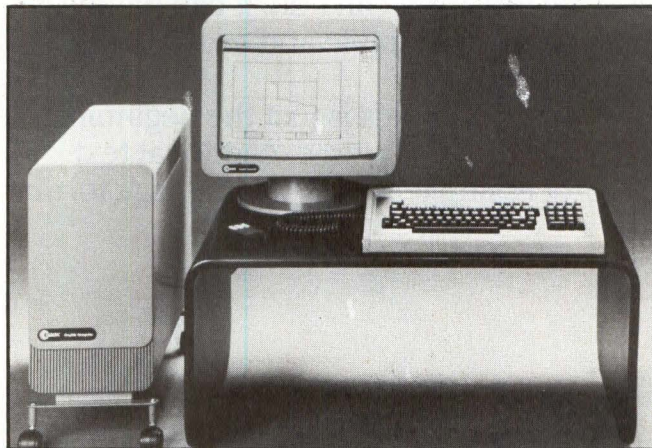
The Cadlink Series 80 allows up to 16 programs to run simultaneously on a single screen—each program having its own screen area.
