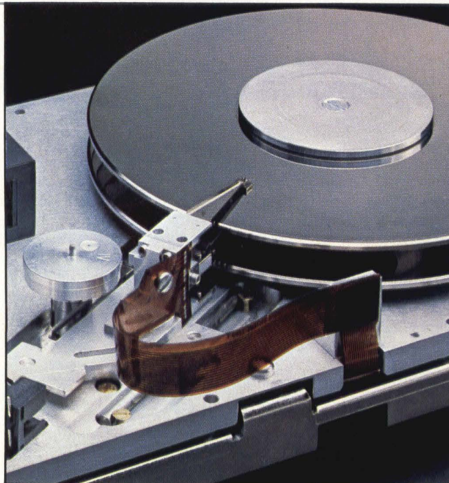
Cogito Systems' Cogitator 912 6M- or 12M-byte half-height 5¼-in. Winchesters use a linear actuator with IBM 3380-type-head-suspension ramp-loaded manganese-zinc read/write heads.
