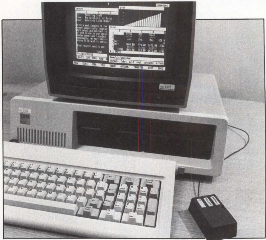
Multiple windows with separate applications can be viewed simultaneously on the same screen with VisiCorp's Visi On package. The product is shown on IBM's Personal Computer, which will be the first system to support the product. The "mouse" at right connects to a standard RS232 port and is used to point to functions and data on the screen.
