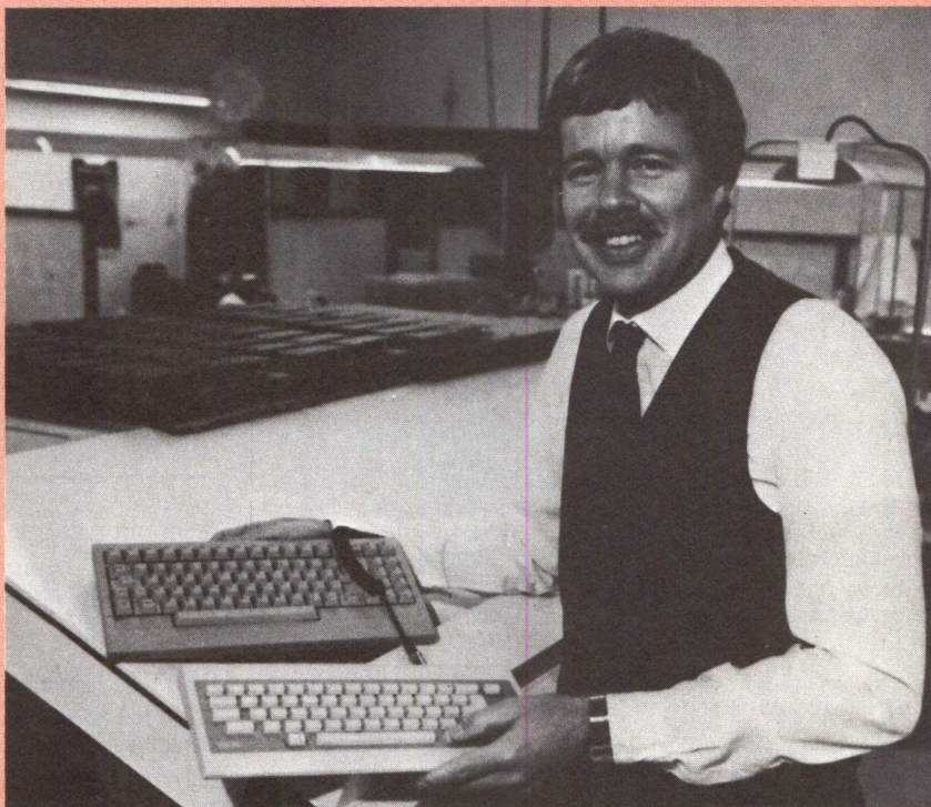
The rectangular shape of keys for the IBM PCjr (lower keyboard) allows enough room between rows to accommodate a bezel template, explains John Overby, president of Advanced Input Devices, which manufactures the keyboard. The flexibility provided by changeable templates is particularly useful in the education market, he says.
