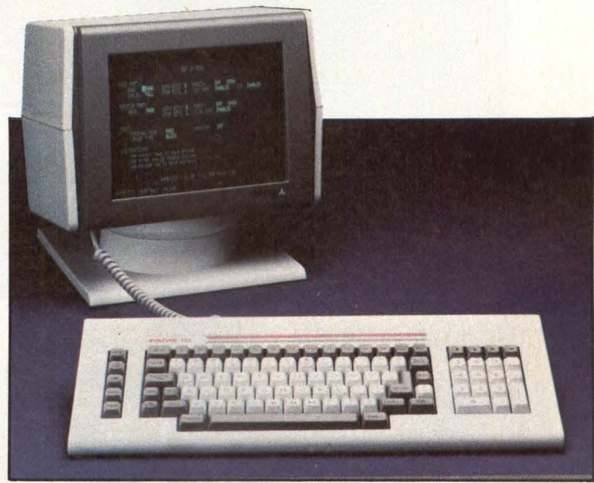
Low in cost but not performance , the $640 Fame III from Falco Data Products typifies the full-featured alphanumeric terminal with a quantity-one price less than $1,000 available to system integrators and OEMs. ANSI X3.64-compatible, it furnishes a soft set-up screen, 12 function keys, three terminal modes, 80-column-by-24-line display and baud rates to 19.2K
