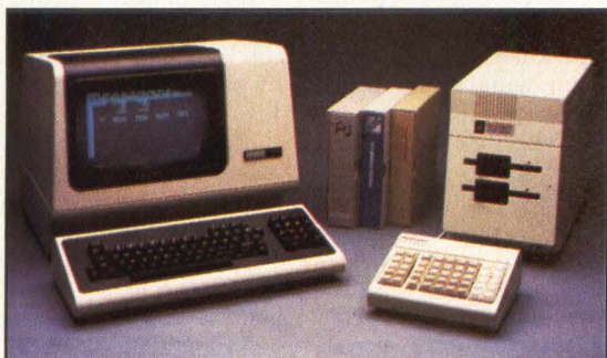
Solaris 1000 running Lotus 123 on a VT-100 type terminal.
