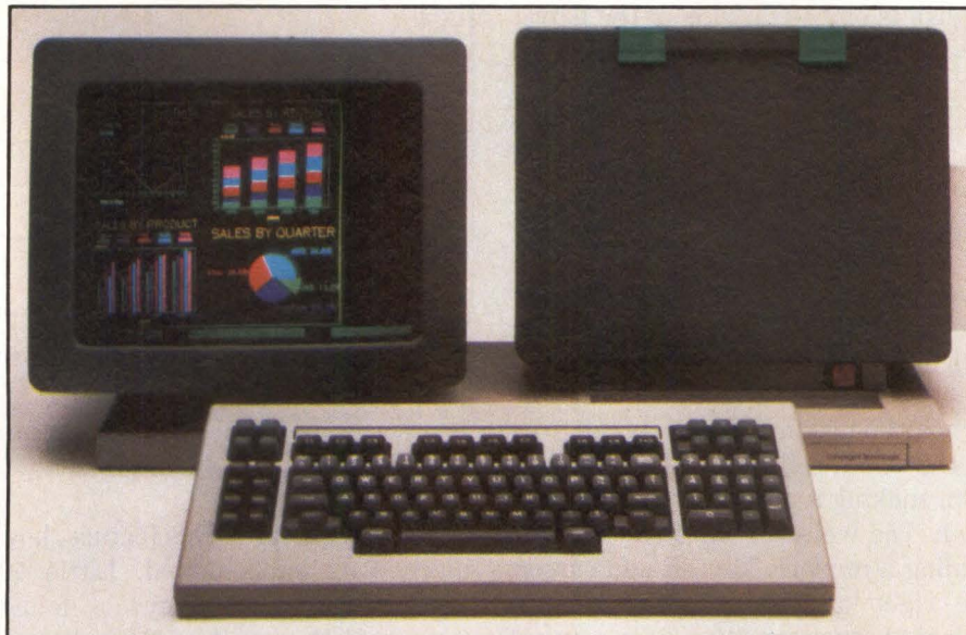
A 15-inch color CRT on a rotating and swiveling socket, and a mainframe enclosure share the AWS workstation's 27-by-9-inch base. The distinctive enclosure contains circuit boards, power supply, a 5M- to 16M-byte Winchester disk and a 5¼-inch floppy-disk drive with as much as 640K of storage.
