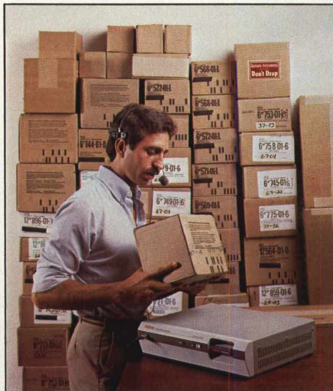
The Verbex 4000 voice-recognition terminal, with a claimed accuracy rate of 98 percent against background noise of 85 dB, is designed for industrial data-entry applications. Not shown is the host IBM PC.
