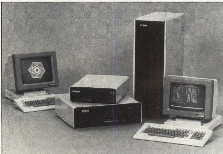
The Stride 400 series from Stride Micro, Reno, Nevada, all contain an identical CPU board with a 10-MHz MC68000 processor. A Corvus Omninet local area network interface is standard.
