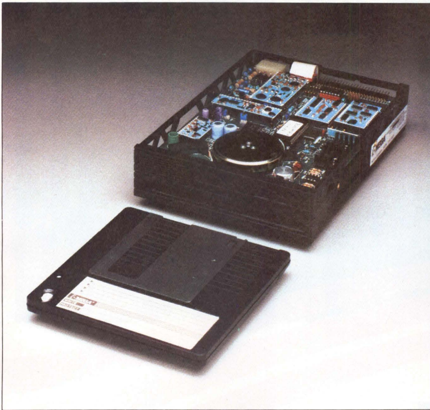
Packing up to 20M bytes into a removable 5 1/4-inch cartridge, the Omega Beta-20 contains an embedded SCSI interface on the master unit and a proprietary interface on the slave module.
