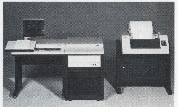
GERMANY'S WUNDERKIND: NIXDORF. Shown is the company's newest offering in the market where German's make their presence felt — small business systems. However, the 8870 is "foreign"-built. The processor comes from Digital Computer Controls, the CRT from Hazeltine, the printer from Dataproducts.
