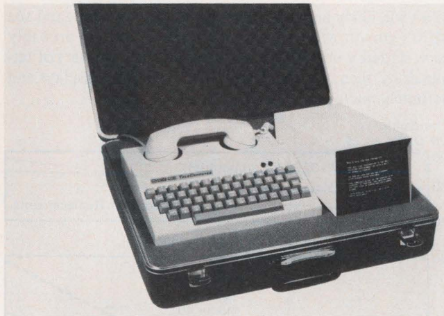
FOR THOSE ON THE MOVE. Digi-Log's portable teletypewriter-replacement type CRT weighs only 23 pounds.
