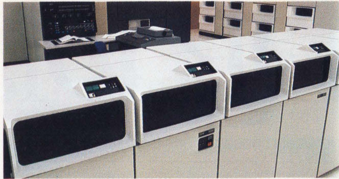
The 3344 and the 3350 contain about twice as much data per square inch as the 3330 Model 11, while for most users the cost per megabyte is typically cut in half.
