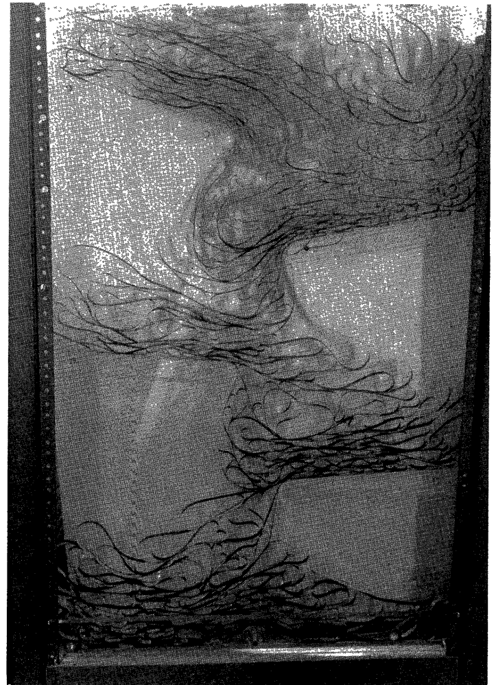
Figure 1. Tape drive unit showing tape supporting projection
