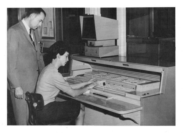
KARD-VEYER ELECTRO-MECHANICAL FILE has a capacity of 80,000 cards. At Aeroquip, it stores miniaturized copies of all the 70,000 engineering tracings turned out by the company since 1940.
