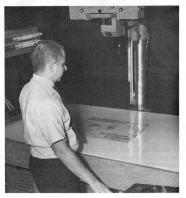
REMINGTON PLANETARY CAMERA is used to take an average of 11 photos of each of approximately 1,000 new and revised tracings a month.
