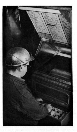
Fig. 5 - IBM 1053 PRINT-OUT TYPEWRITER, located in the same console as the 1713 manual entry unit (at base), reproduces computer instructions at a rate of up to 888 characters a minute.
