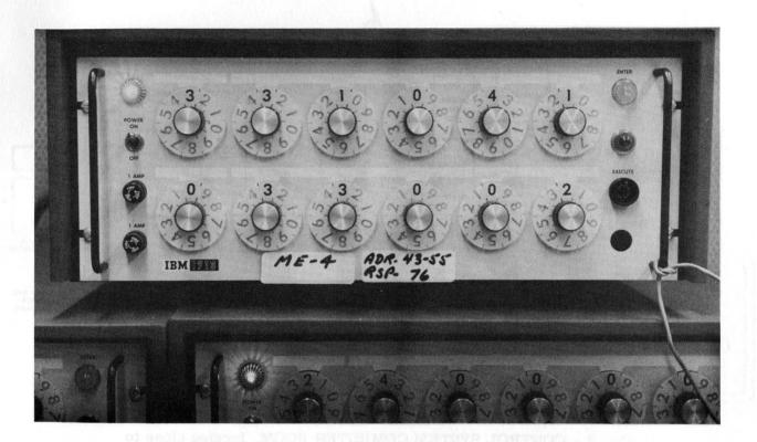
Fig. 4 - IBM 1713 MANUAL ENTRY UNITS, located near furnaces, in the chemistry laboratory and in the shop office, are equipped with 12 rotary switches to permit direct entry of process information and management requests into computer memory.
