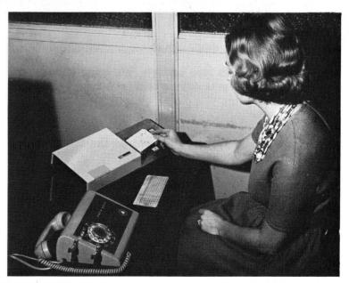
10 IBM 1001 DATA TRANSMISSION UNITS connected to a coast-to-coast private wire network provide punched card order input data.
