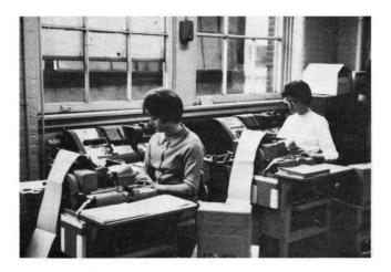
FRIDEN FLEXOWRITER PROGRAMATIC automatic writing machine is the basic unit of the data-origination systems used to produce operation analysis sheets, punched tape records and punched card production travelers.
