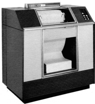
Control Data 168 Arithmetic Unit There are two arithmetic units available with the 160-A — the 168-1 and 168-2. The 168-1 provides fixed point double precision addition and subtraction, plus single or double precision multiply and divide. Arithmetic speeds for the 168-1 are as follows: single precision multiply — 120 \mu sec; single precision divide — 145-180 \mu sec; double precision multiply — 250 \mu sec; and double precision divide — 295-365 \mu sec. Times include obtaining operands from memory and storing the results in memory.
