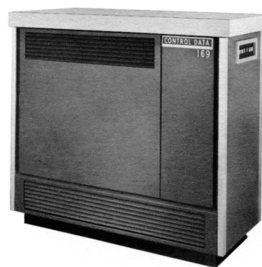
Control Data 169 Auxiliary Memory Unit The Control Data 169 provides expansibility in modules of 8192 12-bit words up to a maximum of 24,576 words of additional external memory. In addition, the 169 provides the option of operating two 160-A Computers together, sharing a common memory and a buffer channel. The additional buffer channels allow I/O operations at a rate of 125,000 words per second.
