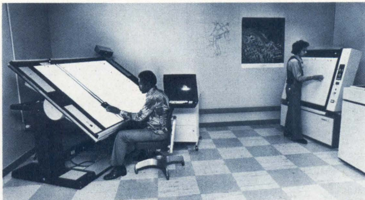
Part of Brooklyn Union Gas mapping system. Input/edit station at left includes digitizing table and CRT display with function and alphanumeric keyboards; high speed plotter is shown at far right
