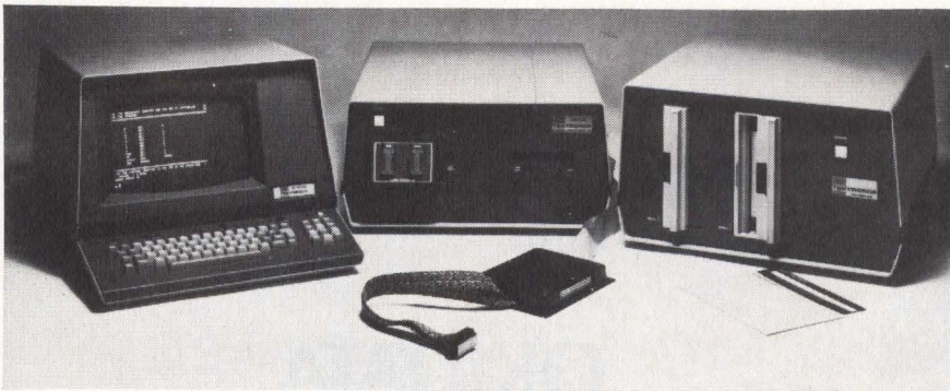
Containing a master memory card, CPU card, disc drive, and disc operating software, Tektronix 8002 is a complete software development aid which also integrates software with the hardware prototype. Both the 8002 and 8001—the in-circuit emulation portion of the system only—currently are designed for use with the 8080 and 6800 microprocessors
