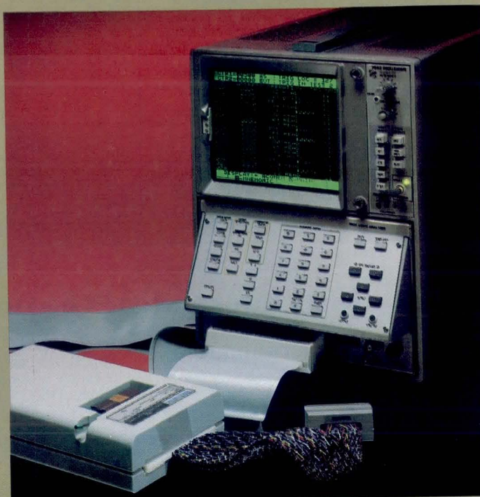
The 7D02 is a 3-wide plug-in for the popular Tektronix 7000 Series oscilloscope. Shown above is a Tek 7603 mainframe housing the 7D02 logic analyzer with a personality module supporting the 6802 microprocessor.
