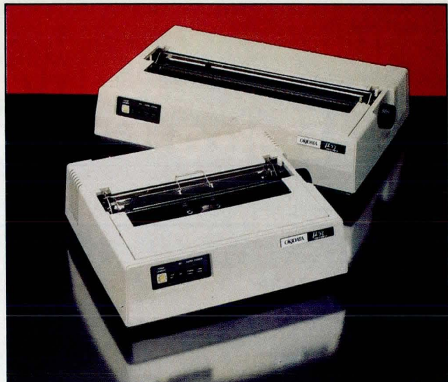
Fig 8 Most dot matrix and full-character impact printers have been packed with useful new features that make them more attractive to the office worker. Besides variable form lengths, speeds, and formats, the units are smaller and lighter due to increased electronics within. Okidata's microline, for example, allows downloading of full-custom character sets from the computer. This makes for faster and more versatile printing.
