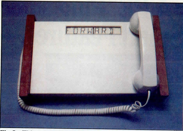
Fig 5 This portable speaker-independent word recognizer designed by Voice Control Systems is a demonstration unit for showing speech recognition capabilities. A liquid crystal display depicts the spoken word, and the telephone handset serves as the microphone.
