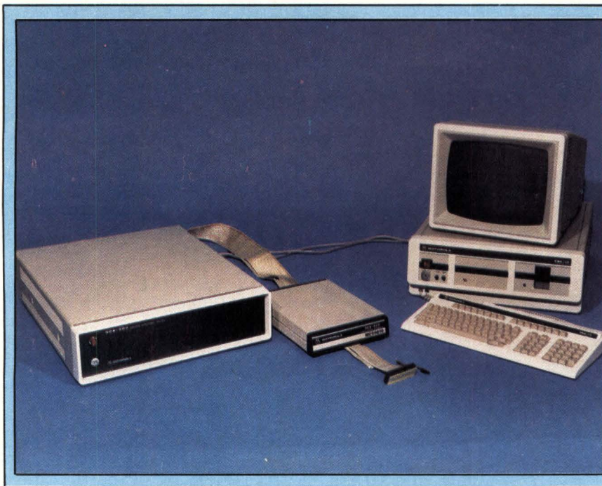
The Unix environment running on the VME/10 workstation from Motorola Semiconductor has been modified to work closely with the HDS 400 hardware station for realtime software debugging.
