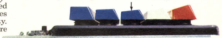
Just .704" (17.88mm) from PC board to keycap top of home row!
