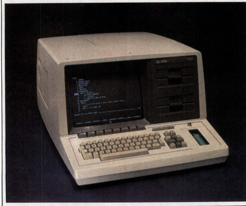
The 64000 workstation from Hewlett-Packard uses a dedicated internal bus to handle peripherals, such as emulators and analyzers, while the control processor and memory reside on a separate bus. This results in increased throughput and realtime measurements.
