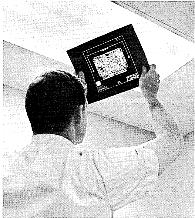
The film positive, made from the negative produced on the plotter, is used as the printing mask for the production of an etched circuit layer in a multi-layer laminate board.
