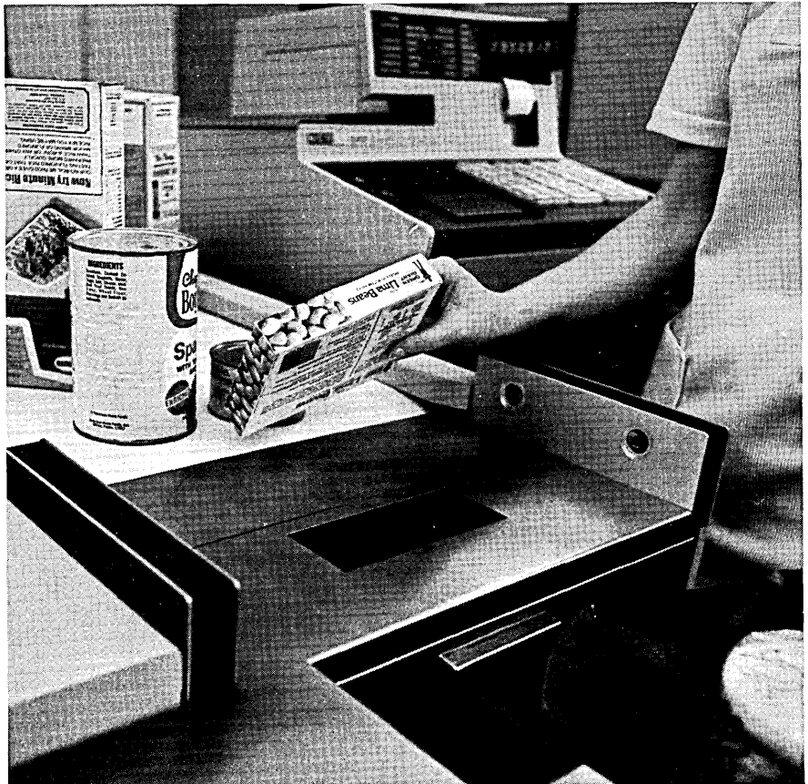
THE UNIVERSAL Product Code can be read at virtually any angle as the item is passed over the scanning window of NCR's electronic checkout system now in operation at a Marsh supermarket in Troy, Ohio. Prices appear on display panels at the top of the Model 255 checkout terminal.
