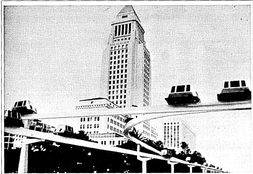
Aerospace Corp. proposed a PRT system for the city of Los Angeles which was to use small, four to six person, cars as illustrated in this photomontage.
