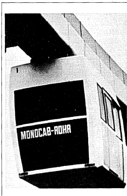
This Rohr vehicle was first shown at Transpo 72, a Washington, D.C., exhibit held by the Urban Transit Administration. Vehicles like this could operate under computer control on a demand responsive schedule.
