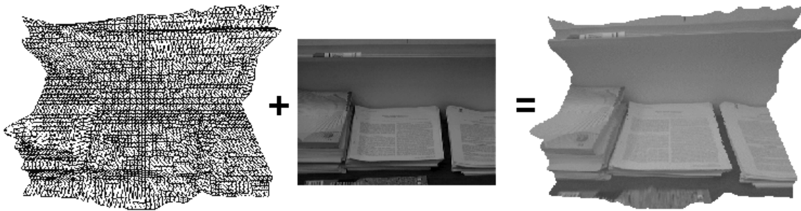
Figure 1: Frontal view of a surface mesh generated from a projective depth map, its corresponding image and the surface mesh with its appearance mapped onto its faces.
