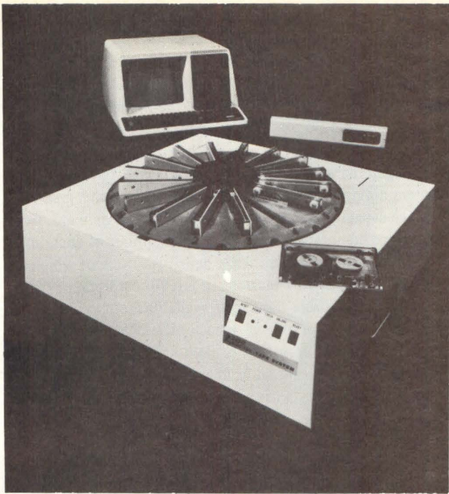
Carousell 5200 , marketed by National Computer Systems, holds up to 16 full-size cartridges for recording digital data.
