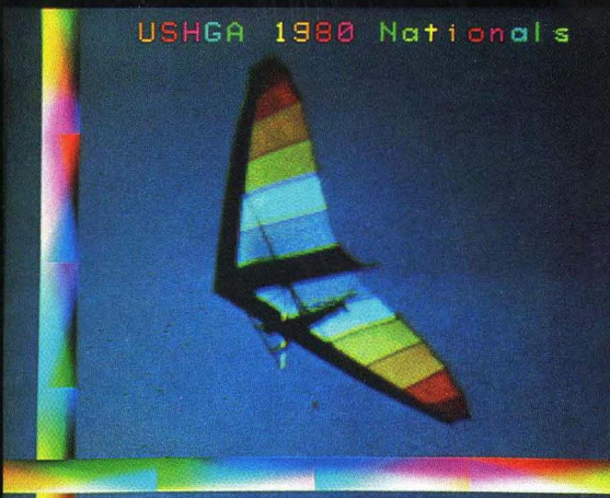
242x256 24-bit pixels, CAT-800, 64K colors. Digitized real color image, 8-bit FRAME GRABBER. Computer generated lettering and color spectrum.
