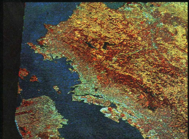
242x256 24-bit pixels, CAT-800, 64K pseudo-colors. LANDSAT infrared image of San Francisco Bay Area.
