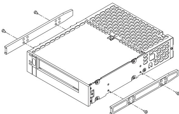
**Figure 5** Attaching slide rails to the tape drive
