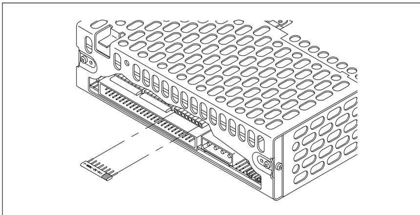
2. Using a pair of flat-nose pliers, carefully grasp each terminator at the center and pull it straight out. Be careful not to squeeze the pliers too tightly or you may break the terminator. Save the unused terminators in case you need to terminate the the bus at tape drive later.
