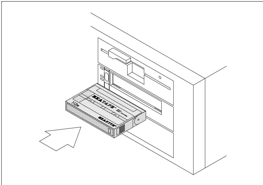
3. Wait while the tape drive loads the tape, determines the tape format, and positions it to the logical beginning of tape (LBOT). This takes about 45 seconds. When the green LED is on solid, the tape drive is ready.
