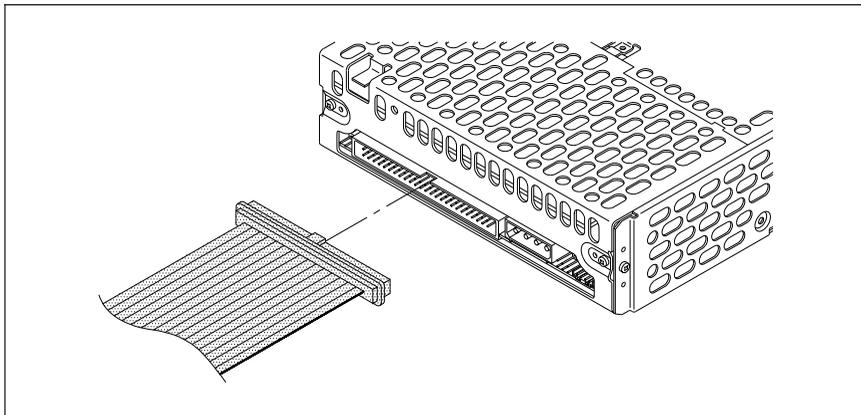
2. From the front of the computer, thread the SCSI ribbon cable into the computer through the open bay.
