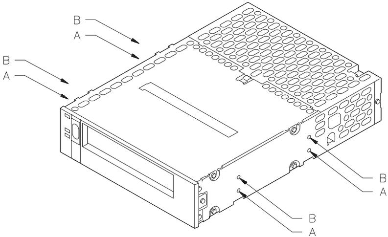
**Figure 14** Mounting holes on the sides of the tape drive
