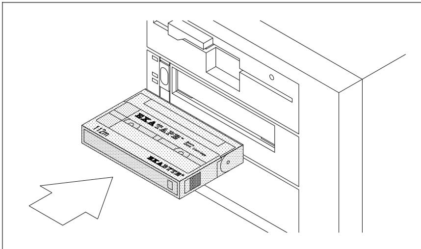
4. The tape drive automatically loads the data cartridge and positions the tape to the logical beginning of tape (LBOT) within approximately 45 seconds (assuming that the data cartridge has already been rewound).
