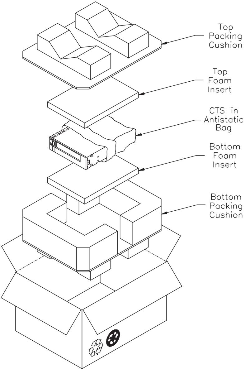
**Figure 12** Single-pack carton and packing materials
