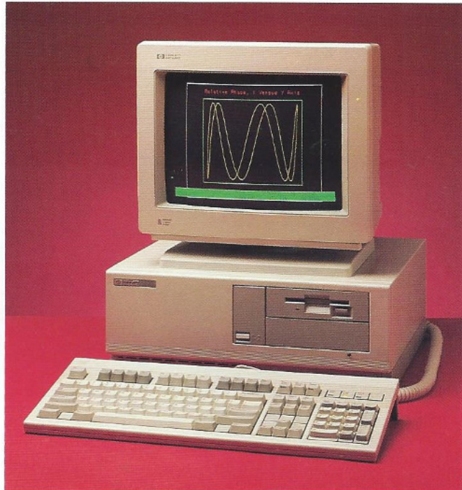
The PC-305CL HP BASIC controller includes an EGA color display and a 20-Mbyte internal hard disc.
