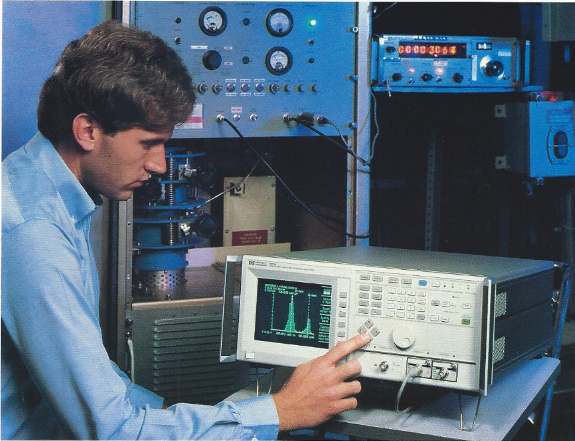
Pulse width jitter, pulse repetition frequency, chirp linearity, and RF pulse rise time can be measured directly with the HP 5371A to simplify radar system characterization.
