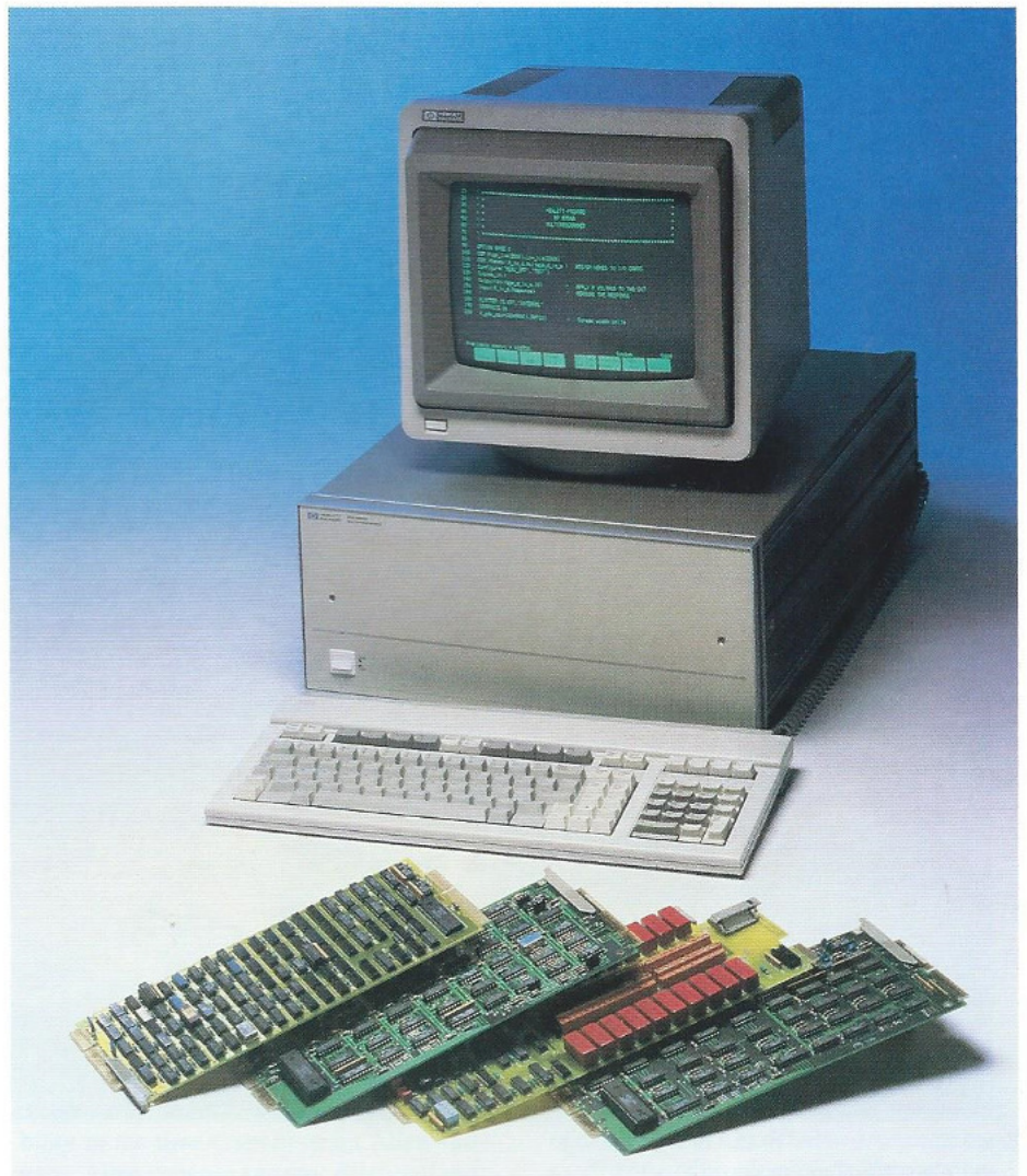
You can adapt a selection of 30 plug-in instrument cards to your specific application needs.
