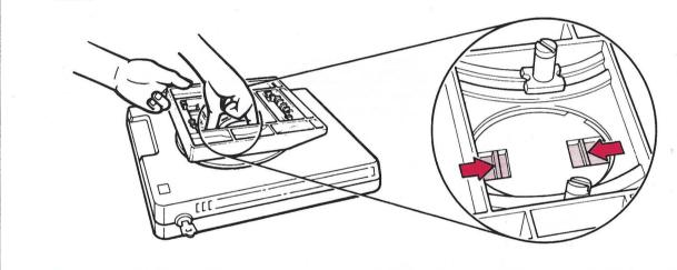
C Lift the stand to make sure it is locked onto the logic element.
