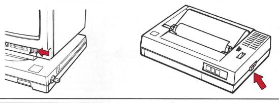
b Insert the printer cable into the connector of the printer and pinch the clamps.
