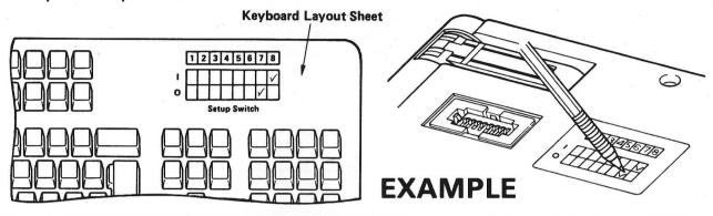
Set the switches as shown on the copy of the keyboard layout sheet. Use a pointed object like a ball point pen. Do not use a pencil.
