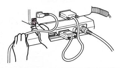
Make sure the distance between the power cord and the video-cable connector is at least 2 centimeters (0.8 inches). Close the cable clamp.
