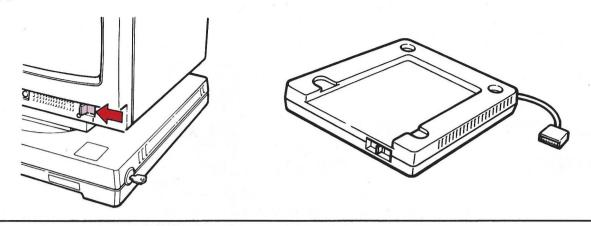
With help from another person, hold the video element as shown and lift the display station onto the expansion unit. (Be careful not to pinch your fingers.)
