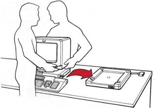
C Insert the expansion unit cable into connector 1 of the logic element and tighten the screws.
