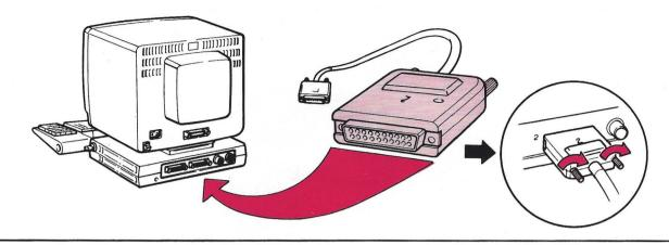
Insert the other end of the video cable into the connector of the video element and tighten screws.
