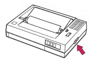
**b** Insert the printer cable into the connector of the printer and pinch the clamps.
