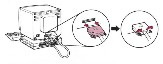
Remove the cap (if present) from the keyboard connector. Insert the keyboard cable into connector 4 and tighten ring by turning it clockwise.
