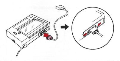
C Insert the other end of the printer cable into connector 1 of the logic element and tighten the screws.
