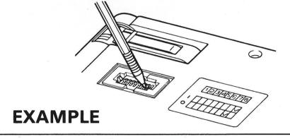
C If specified on the copy of the keyboard layout sheet, change key caps.
