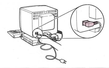
**b** Open the cable clamp and insert the power cord.
