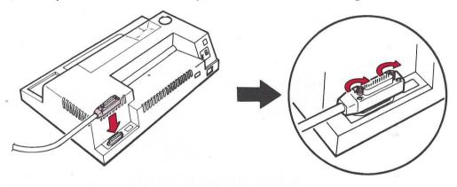
C Insert the cable into connector 8 of the expansion unit and tighten screws.
