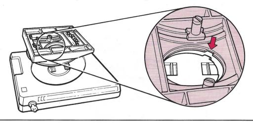
**b** Pinch the two gray latches to lock the stand onto the logic element; then, release them.
