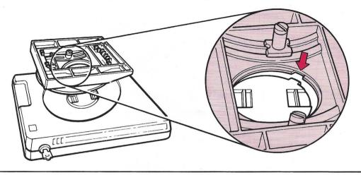
Pinch the two gray latches to lock the stand onto the logic element; then, release them.
