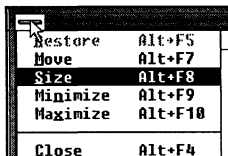
Figure 17-3. A system menu, displayed either when the user clicks the system-menu icon (top left corner) or presses Alt-Spacebar.
