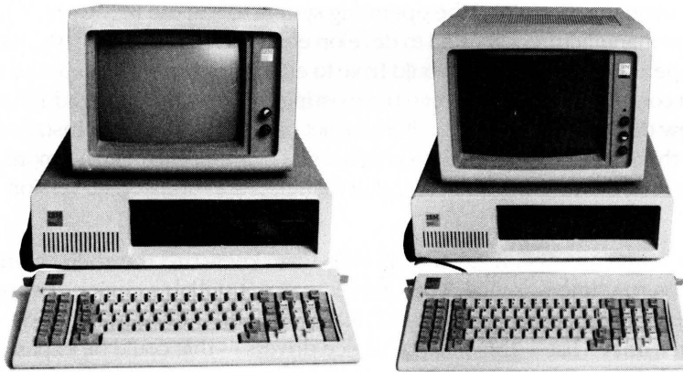
Two members of the IBM line of personal computers for which versions 1 and 2 of MS-DOS were developed. On the left, the original IBM PC (version 1.0 of MS-DOS); on the right, the IBM PC/XT (version 2.0).
